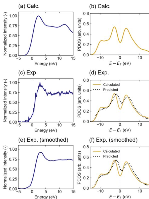
**Figure 6.** (a) DFT-calculated Si-K edge of diamond-type Si. (b) DFT-calculated ground-state PDOS of Si in diamond-type Si. (c) Experimentally obtained Si-K edge of diamond-type Si. (d) Ground-state PDOS predicted from the experimental Si-K edge of diamond-type Si. (e) Smoothed experimental Si-K edge of diamond-type Si. (f) Ground-state PDOS predicted from the smoothed experimental Si-K edge of diamond-type Si.
