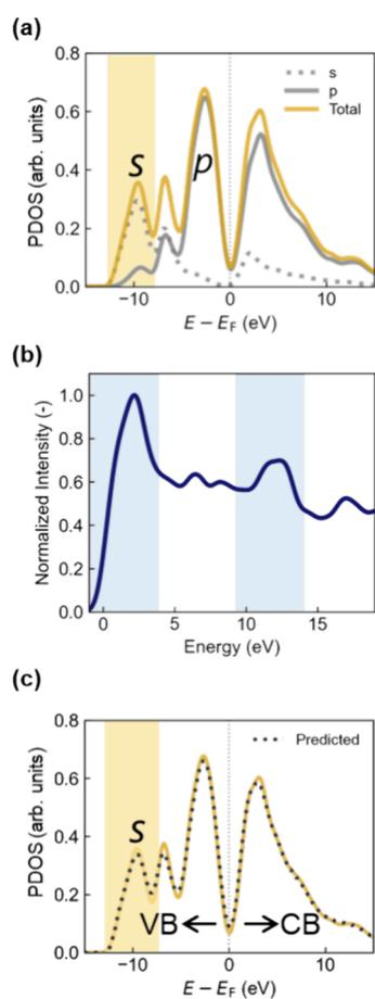
**Figure 1.** (a) Ground-state PDOS of the valence and conduction bands of Si in diamond-type Si calculated by DFT simulation. (b) DFT-simulated Si-K edge in diamond-type Si, where two main peaks can be observed. (c) Result of predicting the ground-state PDOS including both the valence band (VB) and conduction band (CB) of Si atom from the Si-K edge. Fermi level ( $E_F$ ) was aligned to be 0 eV.
