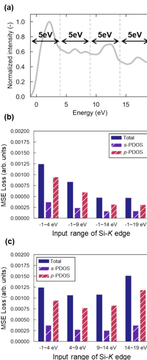
**Figure 3.** (a) Input Si-K edge spectrum, which covers a region of 20 eV, was divided into four sections, each with a range of 5 eV. (b) Change in the MSE as the input region is progressively increased by increments of 5 eV. (c) Variation in the MSE when each 5 eV region is used as an independent input.
