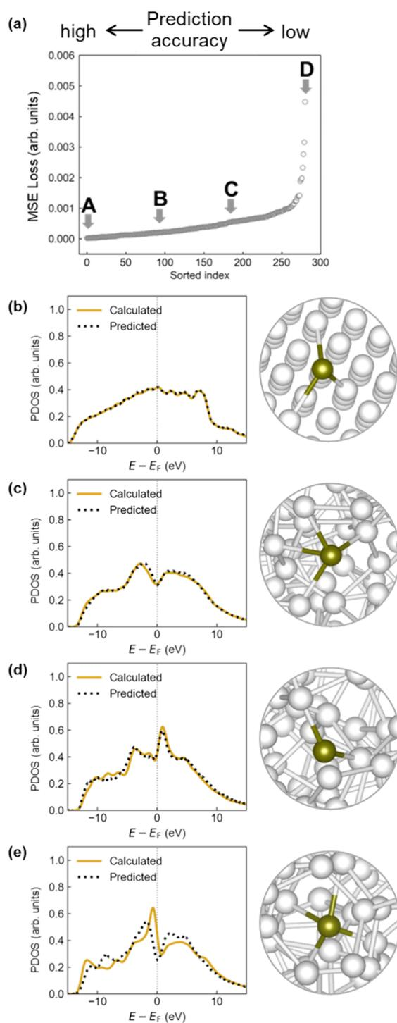
**Figure 2.** Result of prediction for the entire test data set. (a) Sorted mean squared error (MSE) for all the test data. (b) Result exhibiting the highest prediction accuracy among the test data and corresponding local coordination environment around the excited atom (gold). (c) Result corresponding to the top 33% prediction accuracy among the entire test data. (d) Result with top 67% prediction accuracy and (e) worst prediction accuracy.
