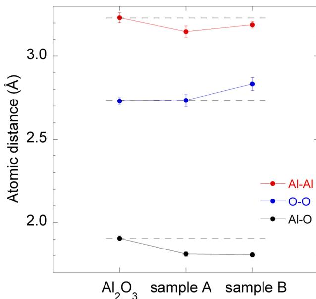
**FIG. 3.** Comparison of the atomic distances of Al–Al, O–O, and Al–O for samples A, B, and Al<sub>2</sub>O<sub>3</sub> polycrystalline. The horizontal broken line is a guide to the eyes for the comparison.
