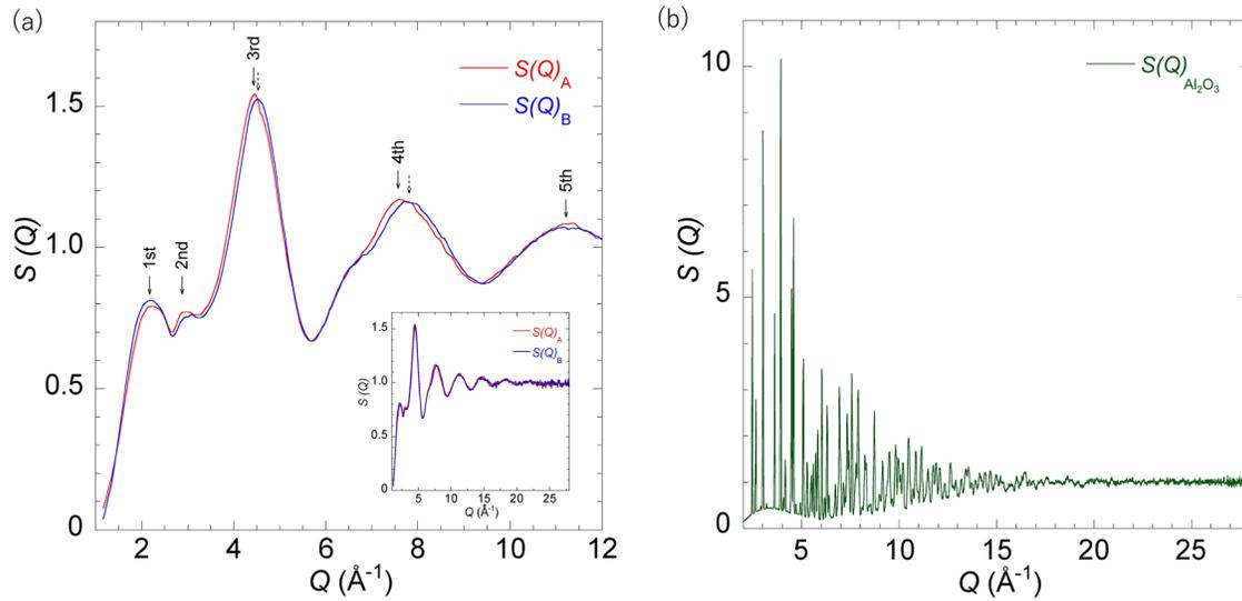
**FIG. 1.** (a) Comparison of the x-ray total structure factor  $S(Q)$  for samples A [ $S(Q)_A$ ] and B [ $S(Q)_B$ ]. The solid (dashed) arrows show the center positions of the profiles for sample A (sample B). The inset shows  $S(Q)_A$  and  $S(Q)_B$  in a whole  $Q$  range. (b) Total structure factor  $S(Q)_{Al_2O_3}$  for  $Al_2O_3$  polycrystalline.
