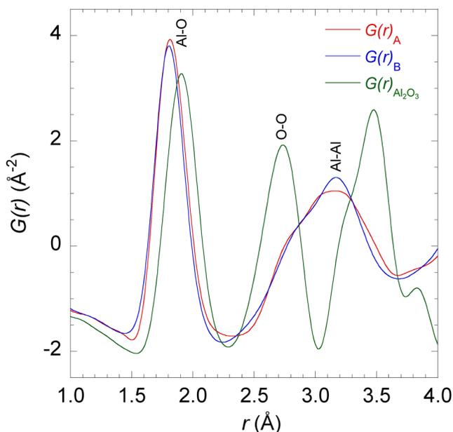
**FIG. 2.** Comparison of reduced PDFs  $G(r)$  for samples A [ $G(r)_A$ ], B [ $G(r)_B$ ], and  $Al_2O_3$  polycrystalline [ $G(r)_{Al_2O_3}$ ].
