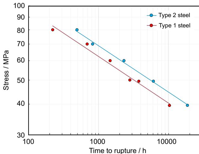
Figure 1: Relationships between stress and rupture time in creep tests at 650°C.
