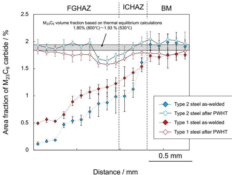
Figure 4: Changes of area fraction of  $M_{23}C_6$  carbides during welding process.
