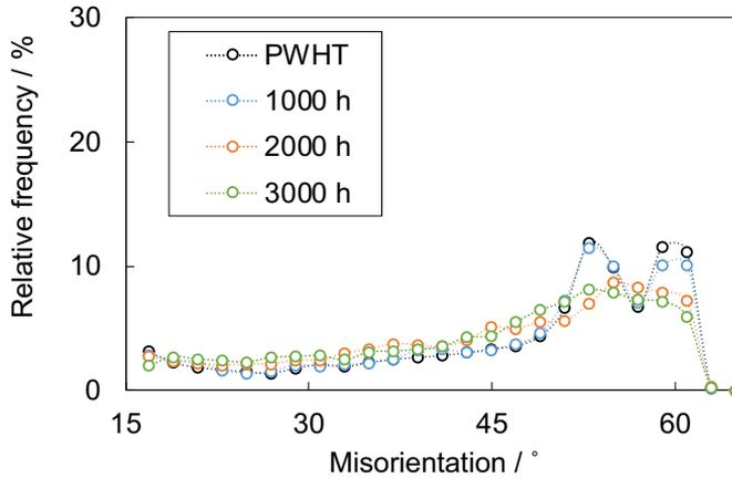
Figure 3: Changes of relative frequency of misorientation during creep test.
