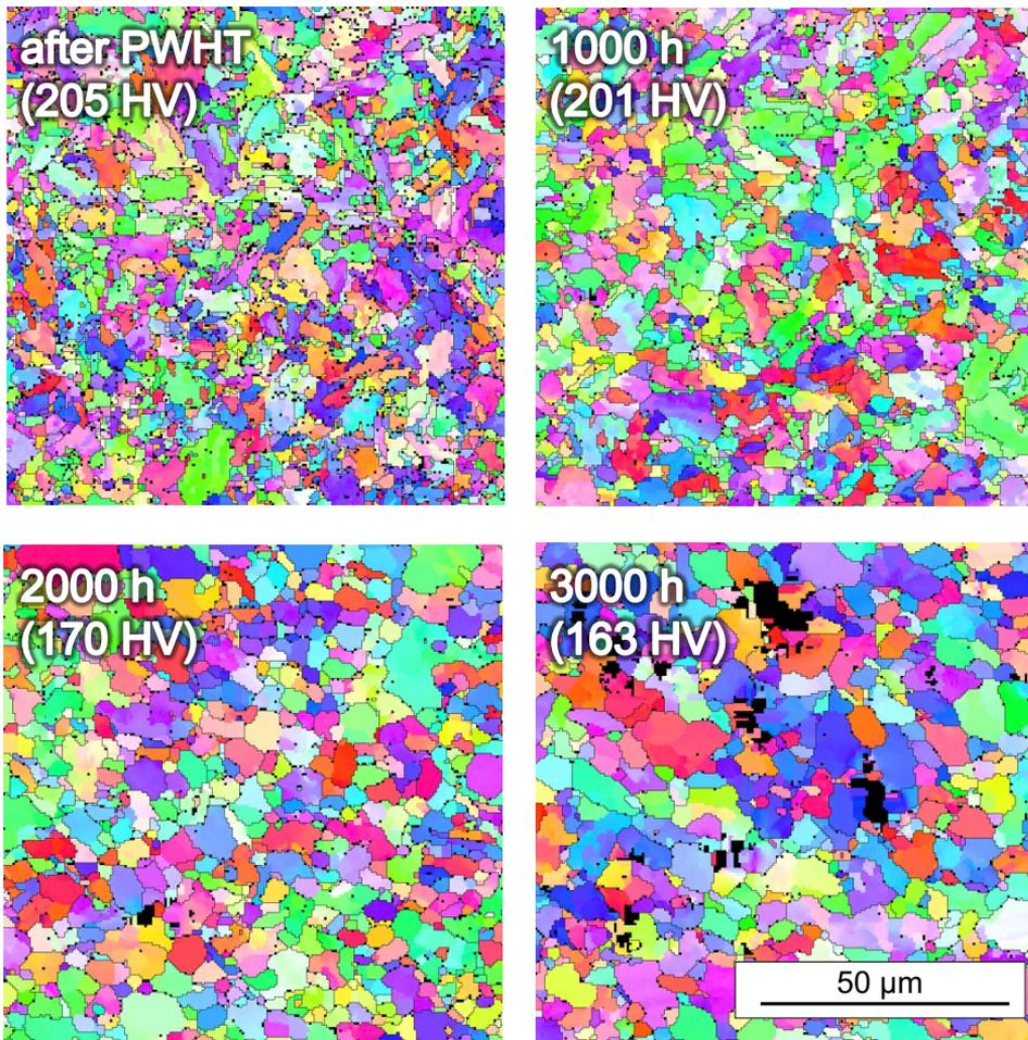
Figure 2: Crystal orientation distribution maps in the FGHAZ of Type 2 steel before and after creep test.
