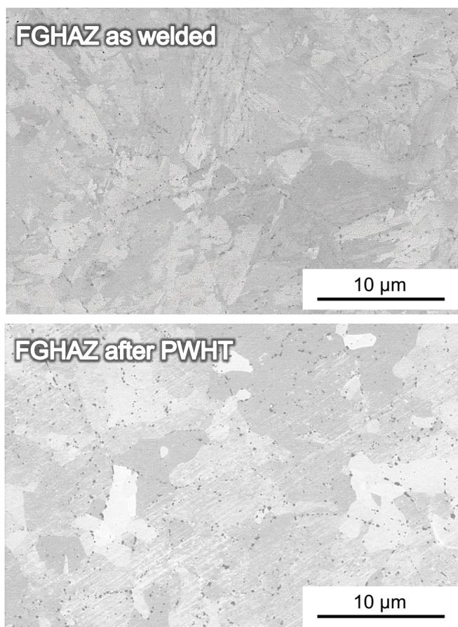
Figure 5: SEM images in the FGHAZ of Type 2 steel as-welded and after PWHT.
