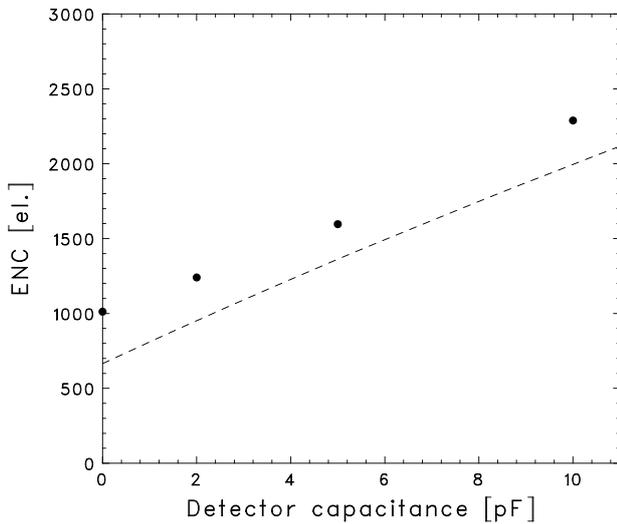
**Figure 7.** Input capacitance versus equivalent noise charges (ENC). The dashed line indicates the SPICE simulation.
