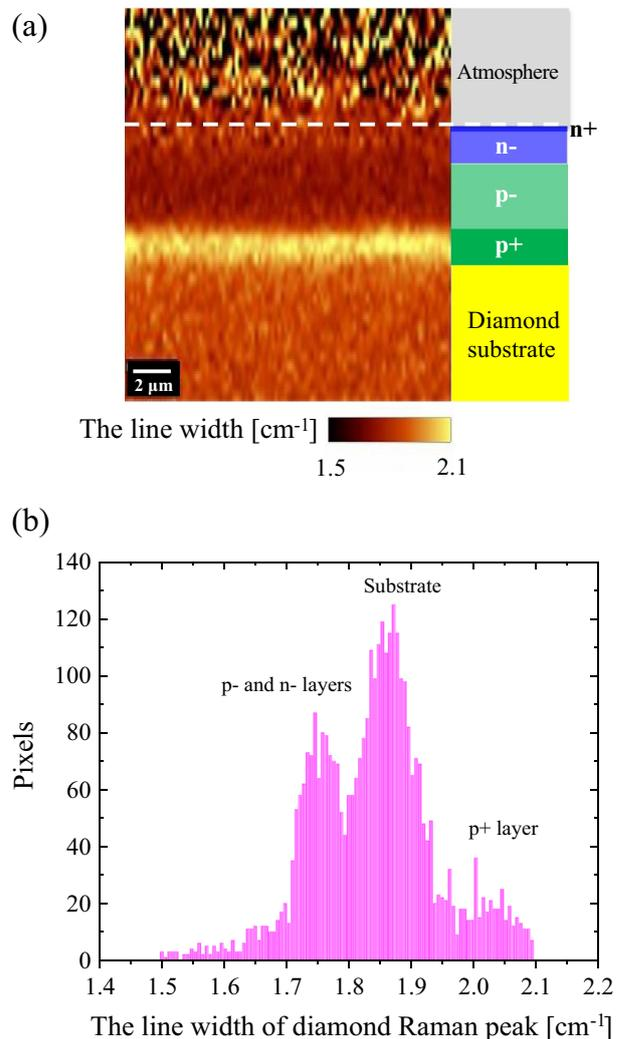
**Figure 4.** (a) Cross-sectional image of the width of the diamond Raman line. The imaging area included the atmosphere and the sample to clear the position of the grown surface. (b) The histogram of the line width in (a).
