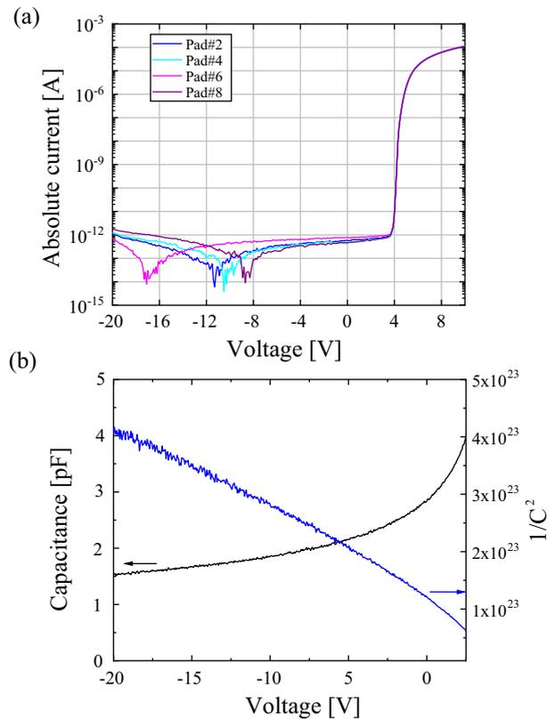
Figure 5. (A) I–V characteristics of the four p–i–n diodes. (b) C–V and  $1/C^2$ –V curves of the p–i–n diode (Pad#2).
