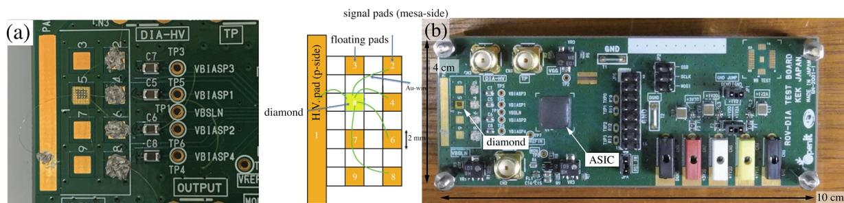
**Figure 8.** (a) Close up image of the diamond sensor and connection to the PCB. (b) Photograph of the dedicated PCB. The readout ASIC was directly mounted on the PCB and molded after wire-bonding.
