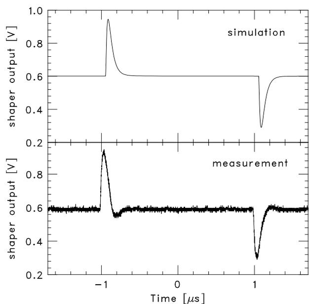
Figure 6. Waveform comparison of the shaper output. A test pulse injects a typical  $\alpha$ -particle event which corresponds to  $\approx 100\text{ke}^-$  into the input.
