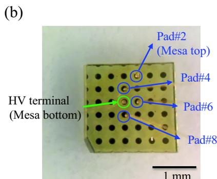
**Figure 2.** (A) Schematic cross-section of a pseudo-vertical p-i-n diode. (b) Optical microscope image of the p-i-n diodes after the wire-bonding. Mesa-top and -bottom were used for the signal output and high-voltage (HV) application, respectively.
