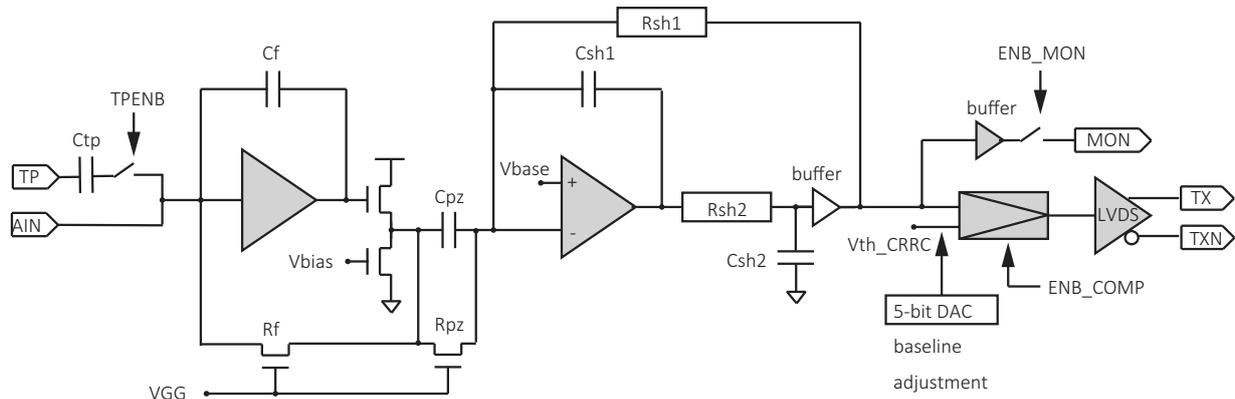
**Figure 3.** Signal processing chain for each channel. The capacitance values are  $C_{tp}=50$  fF,  $C_f=C_{pz}=100$  fF,  $C_{sh1}=35$  fF, and  $C_{sh2}=70$  fF. The resistance values are as follows:  $R_{sh1}=2$  M $\Omega$ ,  $R_{sh2}=150$  k $\Omega$ ,  $R_f$  and  $R_{pz}$  are within the range of several M $\Omega$  adjusted by the gate voltage  $V_{GG}$ .
