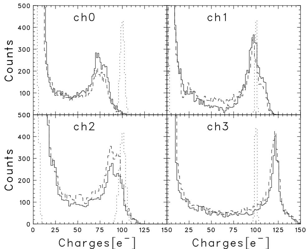
**Figure 9.** Radiation spectra obtained by irradiating 5.48 MeV  $\alpha$ -particles from  $^{241}\text{Am}$ . The reverse voltage of  $-20\text{ V}$  was applied to the p-side of the membrane diamond sensor. The solid and dashed lines indicate the spectra, which were obtained soon after the reverse biasing and after 1 week, respectively. Each exposure time was 20 min. The dotted lines indicate the pedestal and test pulse spectra injected via an on-chip capacitance.
