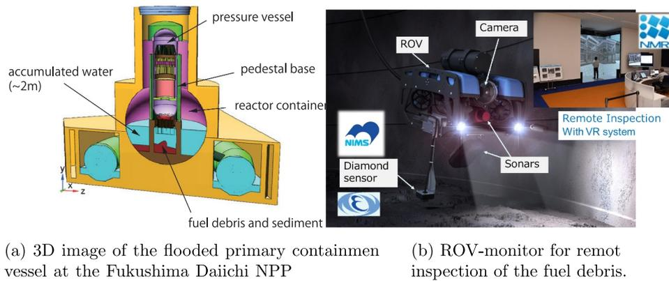
**Figure 1.** (a) 3D image of the flooded primary containment vessel at the Fukushima Daiichi NPP and (b) ROV-monitor for remote inspection of the fuel debris.
