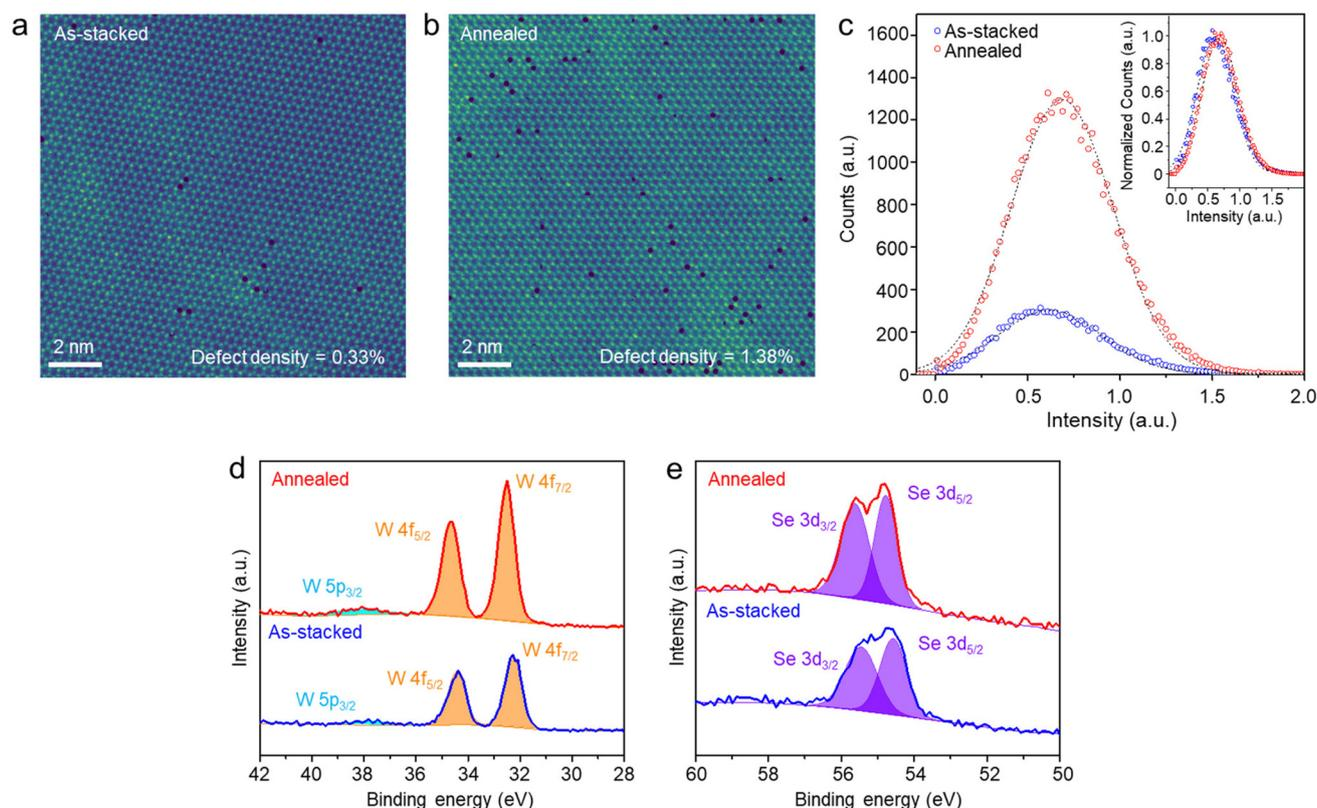
**Fig. 5** Structural analysis of hBN-encapsulated WSe<sub>2</sub> before and after annealing. HAADF-STEM image of graphene-encapsulated 1L-WSe<sub>2</sub> (a) before and (b) after annealing. (c) Spectra of number of defects per total atoms as a function of intensity of defect sites in 1L-WSe<sub>2</sub> before (blue) and after annealing (red). Inset: Normalized Spectra. XPS spectra of (d) W 4f, (e) Se 3d core levels of hBN-encapsulated 2L-WSe<sub>2</sub> before and after annealing.
