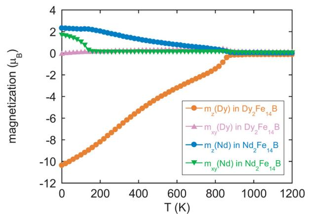
FIG. 3. Temperature dependences of  $m_z(Dy)$  and  $m_{xy}(Dy)$  in  $Dy_2Fe_{14}B$ , and  $m_z(Nd)$  and  $m_{xy}(Nd)$  in  $Nd_2Fe_{14}B$  at the zero field.
