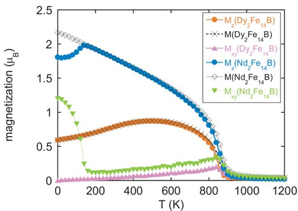
FIG. 2. Temperature dependences of  $M_z$ ,  $M$ , and  $M_{xy}$  at the zero field for  $Dy_2Fe_{14}B$  and  $Nd_2Fe_{14}B$ .
