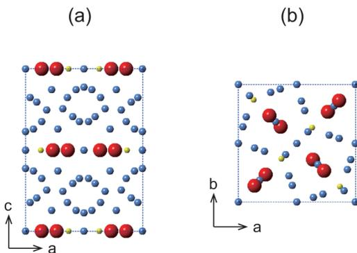
**FIG. 1.** (a) Side view and (b) top view of the unit cell of  $R_2Fe_{14}B$ . R denotes a rare-earth atom (Nd or Dy). In  $Nd_2Fe_{14}B$ ,  $l_a = l_b = 8.80 \text{ \AA}$ , and  $l_c = 12.20 \text{ \AA}$ . In  $Dy_2Fe_{14}B$ ,  $l_a = l_b = 8.76 \text{ \AA}$ , and  $l_c = 12.01 \text{ \AA}$ .
