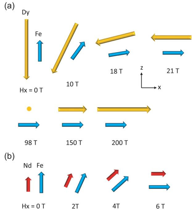
FIG. 8. Alignments of (a) Dy and Fe moments in  $\text{Dy}_2\text{Fe}_{14}\text{B}$  and (b) Nd and Fe moments in  $\text{Nd}_2\text{Fe}_{14}\text{B}$  as a function of  $h_x$ .  $T = 0.46T_c$ .
