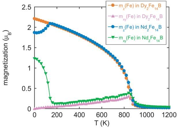
**FIG. 4.** Temperature dependences of  $m_z(\text{Fe})$  and  $m_{xy}(\text{Fe})$  in  $\text{Dy}_2\text{Fe}_{14}\text{B}$ , and  $m_z(\text{Fe})$  and  $m_{xy}(\text{Fe})$  in  $\text{Nd}_2\text{Fe}_{14}\text{B}$  at the zero field.
