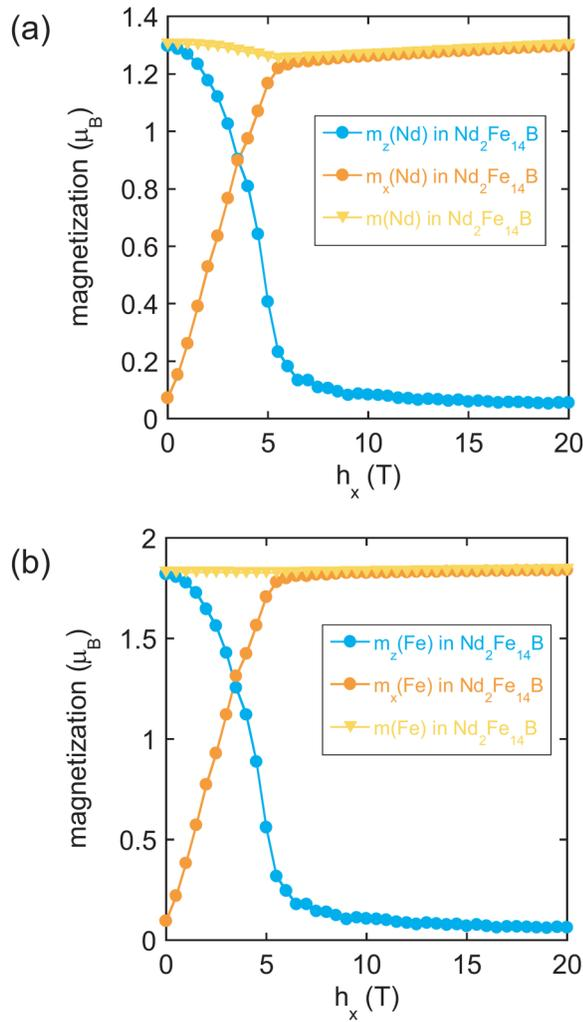
FIG. 7.  $h_x$  dependences of (a)  $m_z(\text{Nd})$ ,  $m_x(\text{Nd})$ , and  $m(\text{Nd})$  and (b)  $m_z(\text{Fe})$ ,  $m_x(\text{Fe})$ , and  $m(\text{Fe})$  in  $\text{Nd}_2\text{Fe}_{14}\text{B}$ .  $T = 0.46T_c$ .
