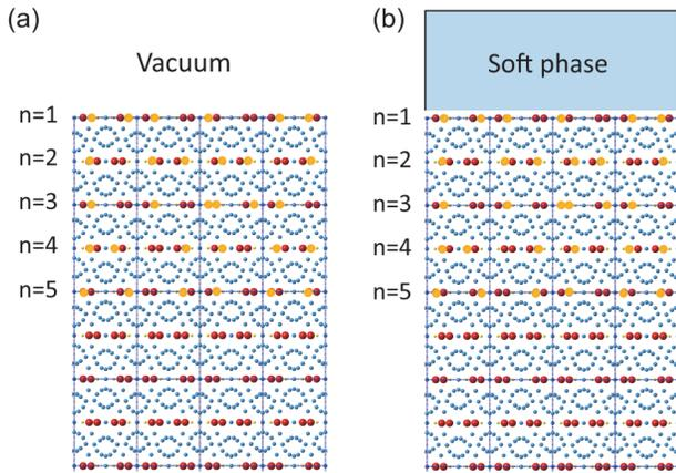
**FIG. 9.** (a) System I. The Nd surface layers are in contact with vacuum. (b) System II. The Nd surface layers are in contact with a soft magnet phase of three-unit-cell thickness. The Nd layers are numbered as  $n = 1, 2, \dots$ . Nd (red) sites are replaced randomly by Dy atoms (orange) with concentration  $P$  between  $n = 1$  and  $n = 5$  and between  $n = 15$  and  $n = 19$ .
