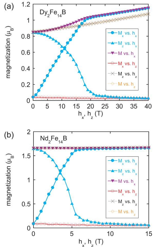
**FIG. 5.**  $h_x$  and  $h_z$  dependences of  $M_x$ ,  $M_z$ , and  $M$  in (a)  $\text{Dy}_2\text{Fe}_{14}\text{B}$  and (b)  $\text{Nd}_2\text{Fe}_{14}\text{B}$ .  $T = 0.46T_c$ .
