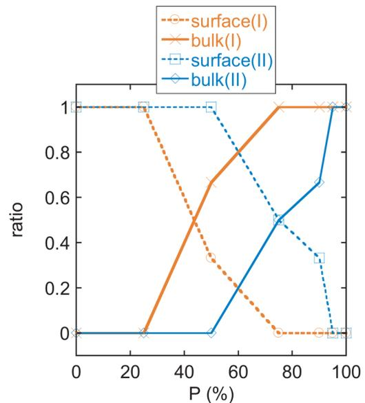
**FIG. 11.**  $P$  dependences of the ratio between the surface and bulk nucleation at  $T = 0.46T_c$  for systems I (dashed line with squares) and II (solid line with circles).
