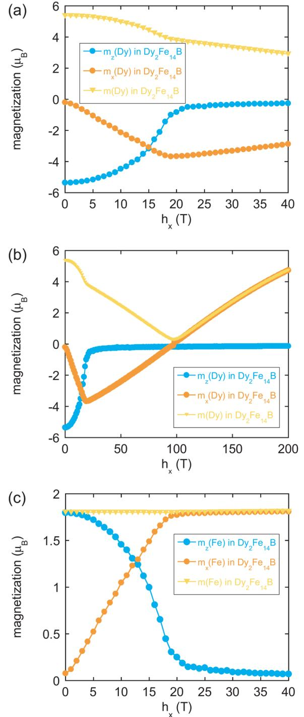
**FIG. 6.**  $h_x$  dependences of  $m_z(\text{Dy})$ ,  $m_x(\text{Dy})$ , and  $m(\text{Dy})$  in  $\text{Dy}_2\text{Fe}_{14}\text{B}$  in (a) a low field range and (b) in a wider field range.  $h_x$  dependences of (c)  $m_z(\text{Fe})$ ,  $m_x(\text{Fe})$ , and  $m(\text{Fe})$  in  $\text{Dy}_2\text{Fe}_{14}\text{B}$ .  $T = 0.46T_c$ .
