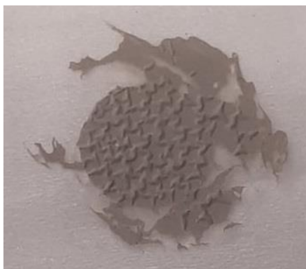
Figure S1. Image of the Grey Si 3 N 4 – 3 sample with wrinkled texture after 2 s exposure.
