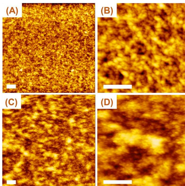
**Figure 3.** (A, B) AFM images of the EP-MSP film obtained at a constant voltage of  $-1.5$  V for 300 s. (C, D) The surface morphology of the EP-MSP film obtained at a constant voltage of  $-1.5$  V for 2000 s. All the scale bars were equal to 500 nm.
