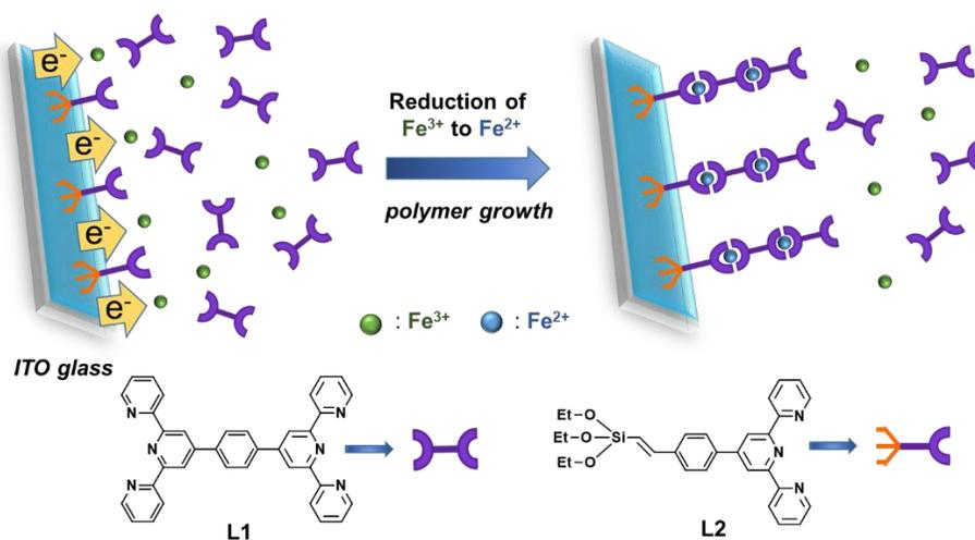
Figure 1. Schematic of the synthesis of electropolymerized MSP (EP-MSP)-thin film containing Fe<sup>2+</sup> ions, a "connecting ligand" (**L1**), and a "bridging ligand" (**L2**) on an ITO glass
