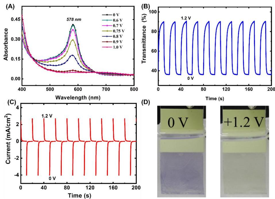
**Figure 4.** (A) In-situ UV-vis spectra of EP-MSP film in a 0.1 M LiClO<sub>4</sub>/ACN solution at different applied potentials. (B) Transmittance change ( $\Delta T$ , %) at 578 nm of EP-MSP film switched between 0 and +1.2 V in 0.1 M LiClO<sub>4</sub>/ACN with an interval time of 10 s. (C) In-situ current response in the EP-MSP film when switching between 0 and 1.2 V. (D) Digital pictures of EP-MSP film color switching.
