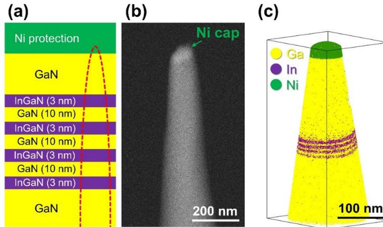
**Figure 4.** The demonstration of the automatic “site-specific” tip preparation from the InGaN-based MQWs with the Ni protection cap. (a) The schematic of the sample structure. (b) The SEM image of the prepared tip in which Ni was intentionally kept at  $\sim 50$  nm. (c) The obtained 3D atom map from the tip.
