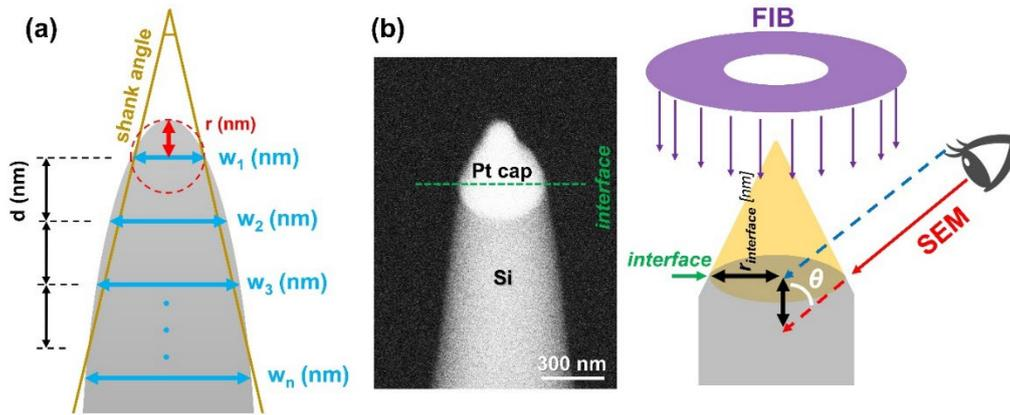
**Figure 2.** Definition of tip shape. (a) Schematic of the tip shape defined by the radius of curvature and the shank angle. (b) A typical TLD-BSE image of the Pt-capped Si needle during the FIB sharpening process. The coincidence angle  $\theta$  of FIB and SEM should be considered to determine the interface position.
