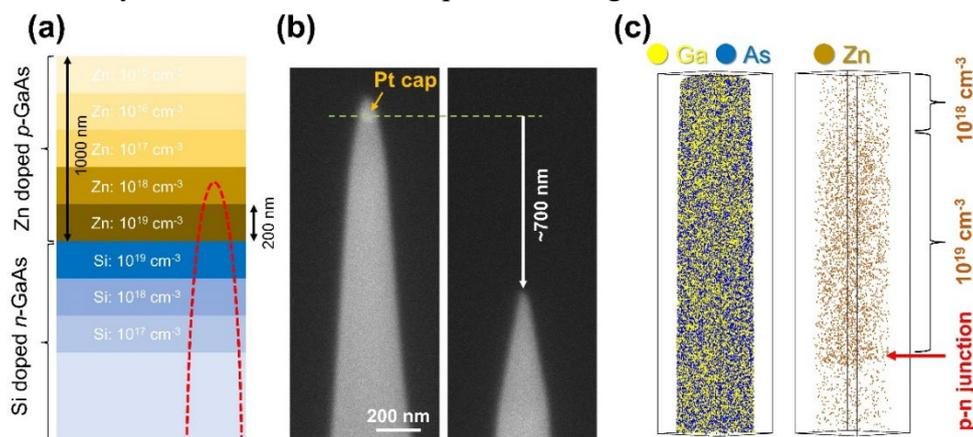
**Figure 5.** The automatically prepared tip from a  $p$ - $n$  junction of GaAs. (a) The schematic of the sample structure. The  $p$ - $n$  junction is located at a depth of 1,000 nm from the surface. (b) The final tip with the top  $\sim 700$  nm was removed. (c) The obtained 3D atom map of Ga, As, and Zn.
