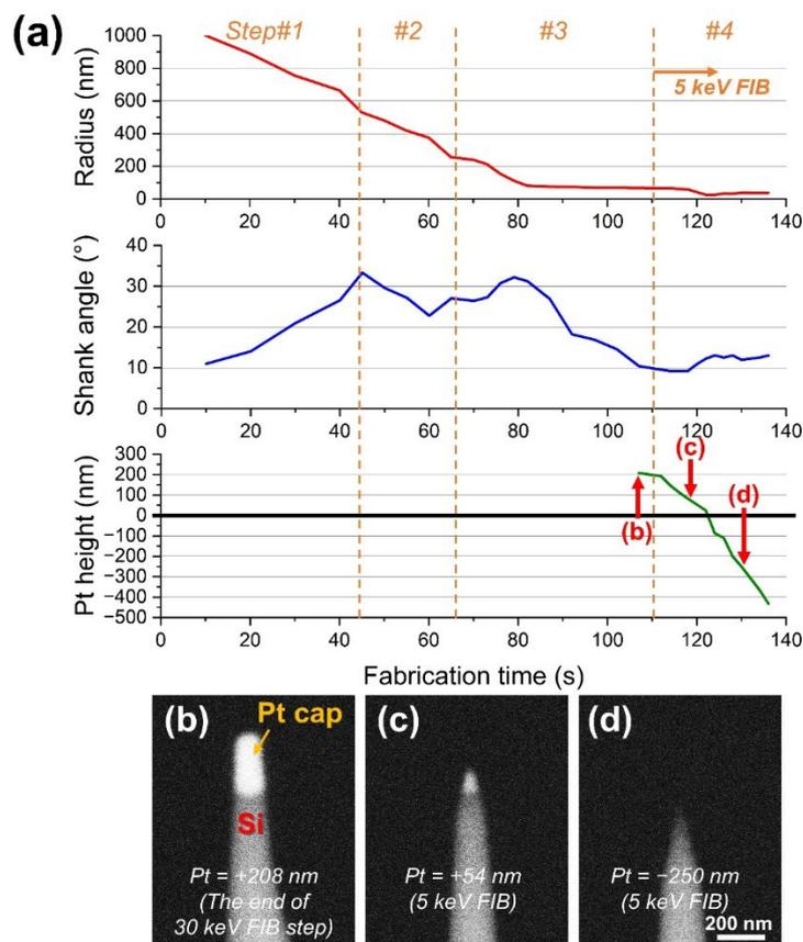
**Figure 3.** Demonstration of how the automated tip preparation program works. (a) Monitored tip radius, shank angle, and the remained Pt height as a function of FIB fabrication time. Here, the target Pt height was set as -400 nm to show how the program works. (b) The Si tip at the end of 30 keV (step 4 in Table 1). (c) The tip with 54 nm Pt cap remaining. (d) The Si tip after the Pt protection is completely removed by the low keV FIB cleaning.
