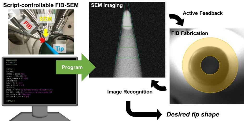
**Figure 1.** Schematic of an automated tip fabrication using a script-controllable FIB/SEM system. Run the Python-based program on a script-controllable FIB/SEM, then repeat tip shape monitoring using an SEM image and active feedback FIB fabrication until the tip has the desired shape.
