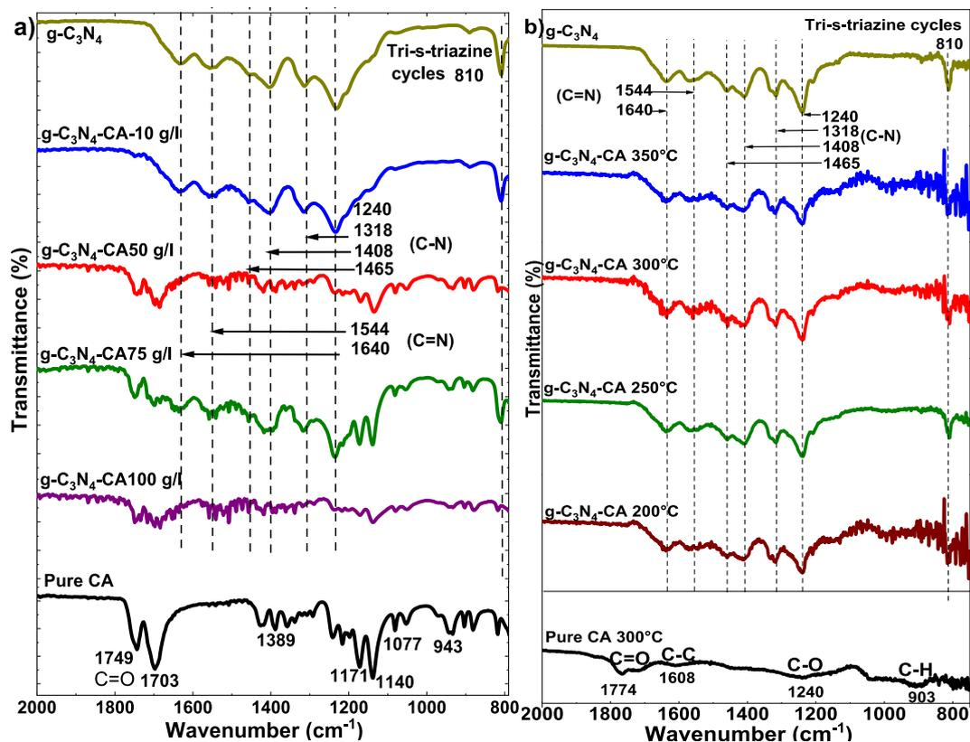
**Fig. 4.** FTIR of  $g\text{-C}_3\text{N}_4$  and  $g\text{-C}_3\text{N}_4\text{-CA}$  on ITO glass obtained at a) by varying the CA concentration, without additional heat treatment, and b) various calcination temperatures at 200–350 °C.
