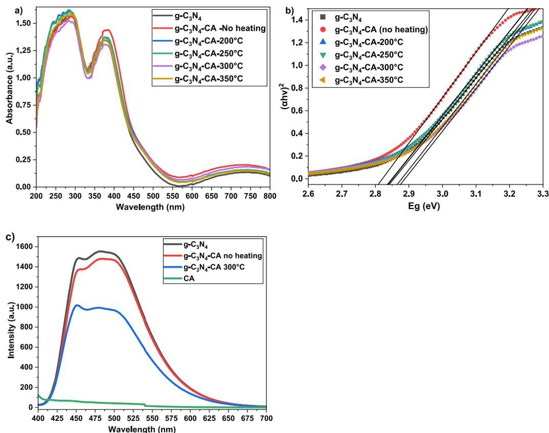
**Fig. 6.** UV-vis spectra of  $g\text{-C}_3\text{N}_4\text{-CA}$  on ITO glass obtained at a) different calcination temperatures, with a constant CA concentration of 75 g/l, b) band gap energy of the thin films and c) photoluminescence (PL) spectra of  $g\text{-C}_3\text{N}_4$  and  $g\text{-C}_3\text{N}_4\text{-CA}$  on ITO glass before and after heating at 300 °C.
