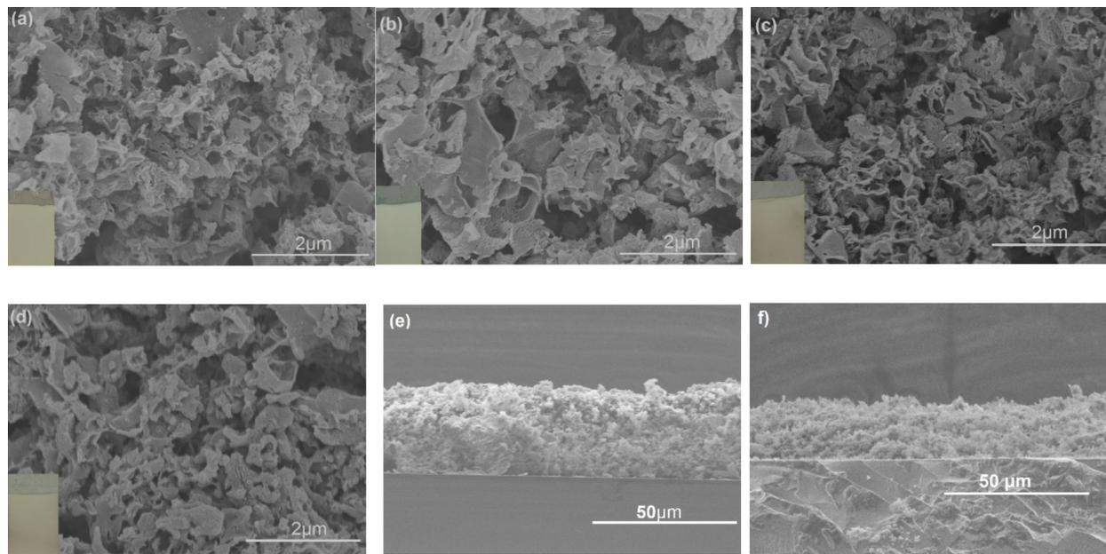
Fig. 2. FE-SEM images of EPD films containing a)  $g\text{-C}_3\text{N}_4$  and b)  $g\text{-C}_3\text{N}_4\text{-CA}$  c)  $g\text{-C}_3\text{N}_4\text{-CA}$  200 °C d)  $g\text{-C}_3\text{N}_4\text{-CA}$  300 °C, Cross-section of e)  $g\text{-C}_3\text{N}_4$  f)  $g\text{-C}_3\text{N}_4\text{-CA}$ -300 °C, with a constant CA concentration of 75 g/l.
