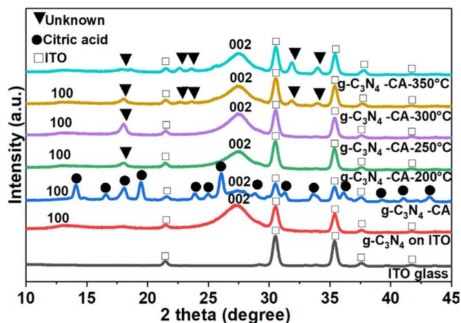
Fig. 3. X-ray diffraction (XRD) patterns of the films on ITO glass obtained at different calcination temperatures with a constant CA concentration of 75 g/l.
