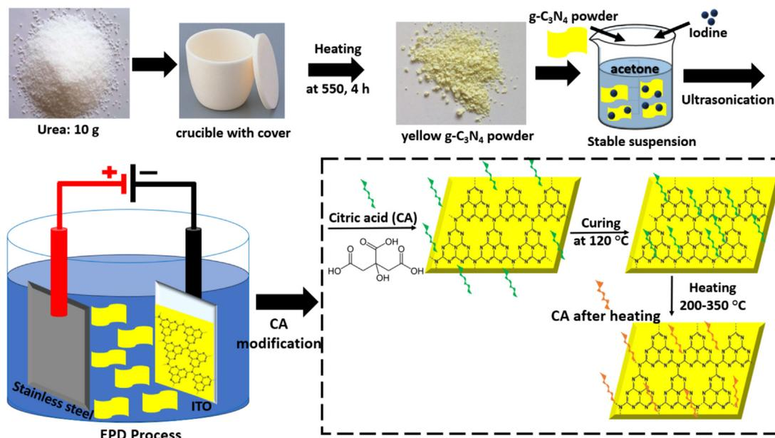
Fig. 1. Schematic overview of CA modified  $g\text{-C}_3\text{N}_4$  film fabrication via thermal process.
