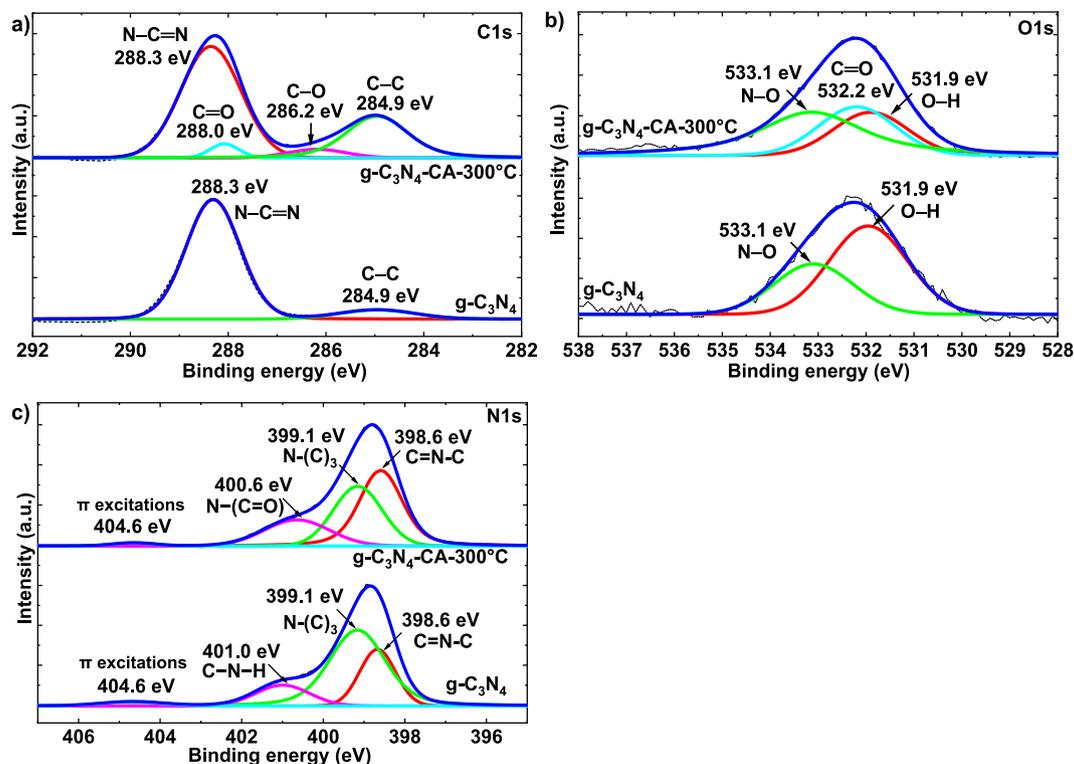
Fig. 5. XPS spectra of  $g\text{-C}_3\text{N}_4$  and  $g\text{-C}_3\text{N}_4\text{-CA-300 } ^\circ\text{C}$ .
