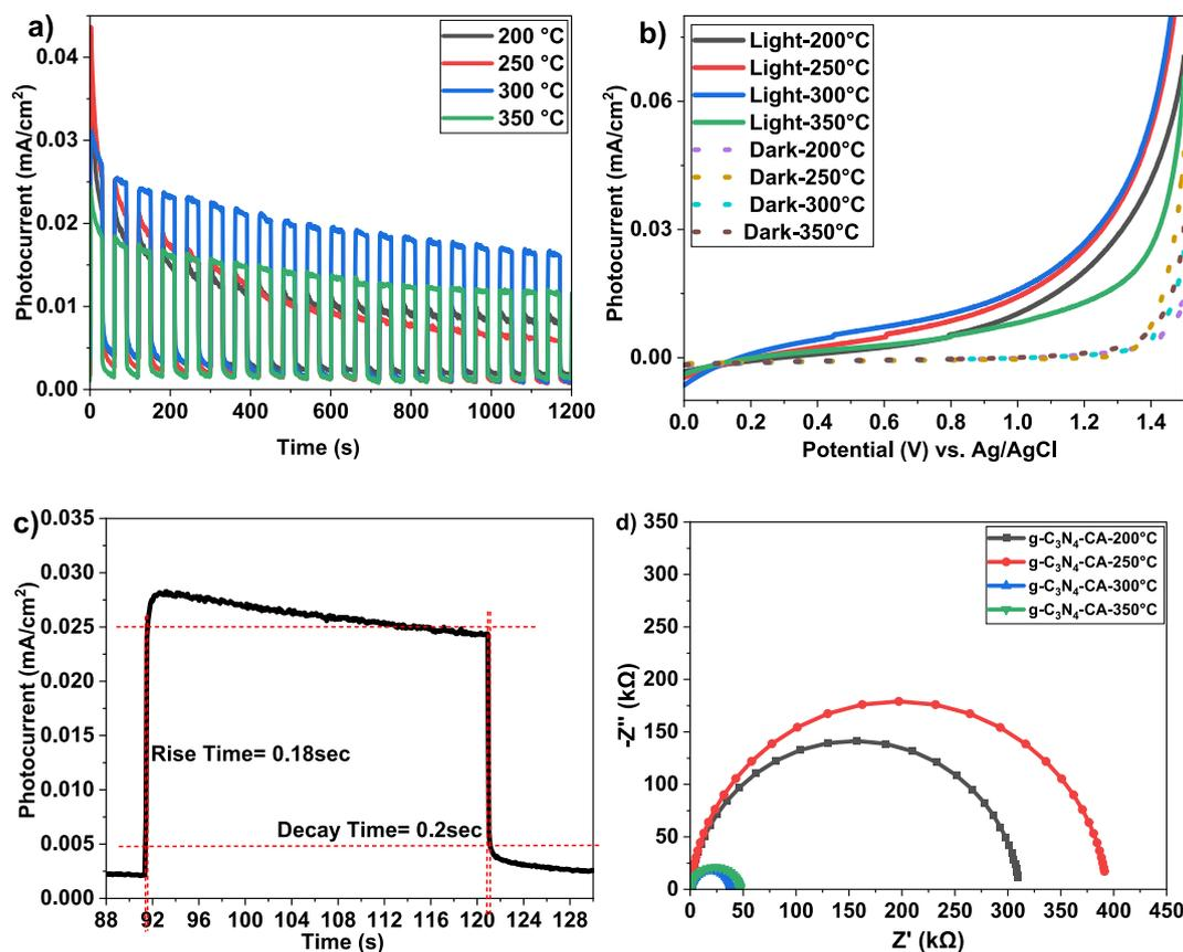
**Fig. 7.** A) photocurrent response, b) linear sweep voltammetry (LSV) plots of the films at different calcination temperatures, c) enlarged rising and decaying edges of the photocurrent response of the  $g\text{-C}_3\text{N}_4\text{-CA-300 °C}$ , and d) EIS Nyquist plots of citric acid-modified  $g\text{-C}_3\text{N}_4$  films.
