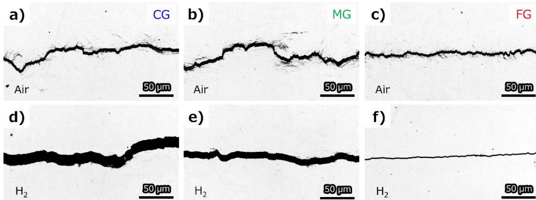
Fig. S2 Optical micrographs around the lateral surfaces of CT specimens of (a)(d) CG, (b)(e) MG, and (c)(f) FG in (a)~(c) air and (d)~(f) 90 MPa  $\text{H}_2$  gas. The relevant  $\Delta K$  is  $15 \text{ MPa}\cdot\text{m}^{1/2}$ , and the crack growth direction is from left to right in each image.
