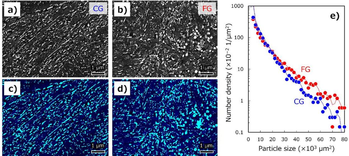
Fig. S1 (a)(b) SEM images of the microstructures in (a) CG and (b) FG after etched with picric acid, wherein cementite precipitates are appeared as white particles. The relevant bipolarized images are depicted in (c) and (d). (e) presents the number density histograms of particle sizes, constructed from the analysis of SEM images containing more than 20000 particles for each material.
