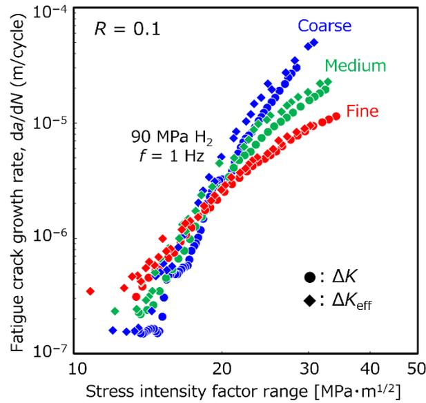
Fig. S3 Fatigue crack growth rates of CG, MG, and FG in 90 MPa  $\text{H}_2$  gas assembled versus apparent stress intensity factor range,  $\Delta K$ , and effective stress intensity factor range,  $\Delta K_{\text{eff}}$ . For the determination method of  $\Delta K_{\text{eff}}$ , the readers shall refer to [34].
