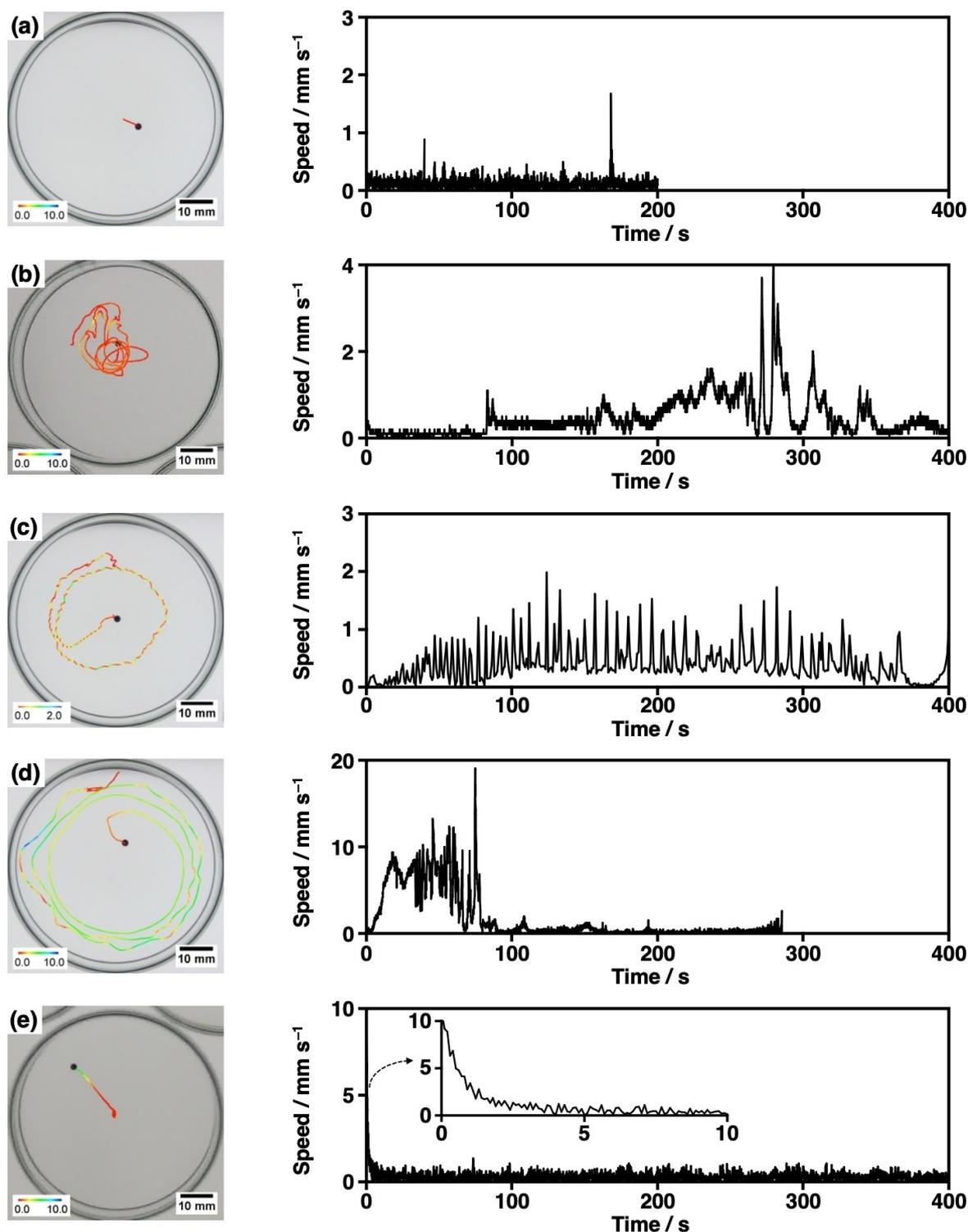
**Figure 3.** Top view of the trajectory (left) and speed profile (right) of **PDI 1** disks on a CHES buffer solution containing various concentrations of  $\text{Na}_2\text{S}_2\text{O}_4$ : (a) 2.3 mM, (b) 11 mM, (c) 23 mM, (d) 46 mM, and (e) 92 mM. The color of the trajectory indicates the speed of the disk in  $\text{mm s}^{-1}$ .
