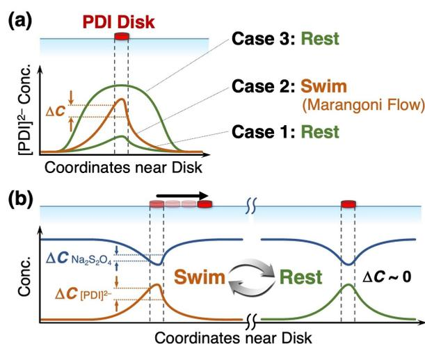
**Figure 4.** (a) Schematic diagram depicting three  $[\text{PDI}]^{2-}$  concentration profile scenarios. (b) Mechanism of the oscillatory motion of PDIs on water upon reduction.
