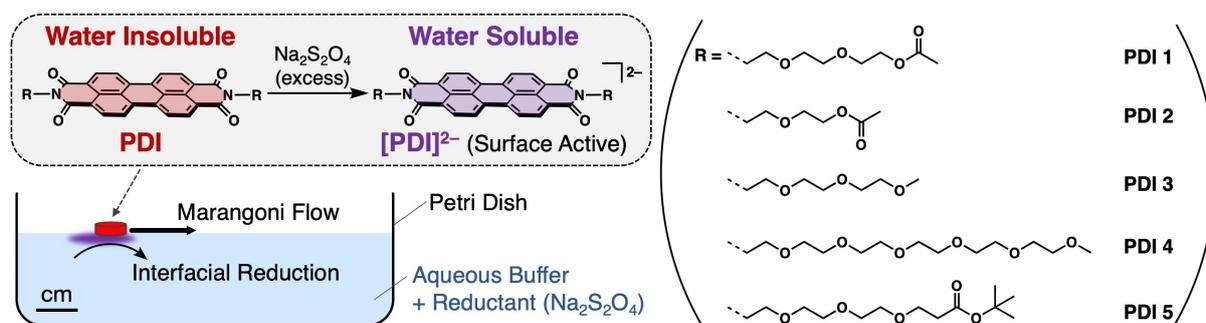
**Figure 1.** Schematic illustration of the reduction reaction of **PDI 1–5** at the water surface to form their dianion counterparts, which induces Marangoni flow.
