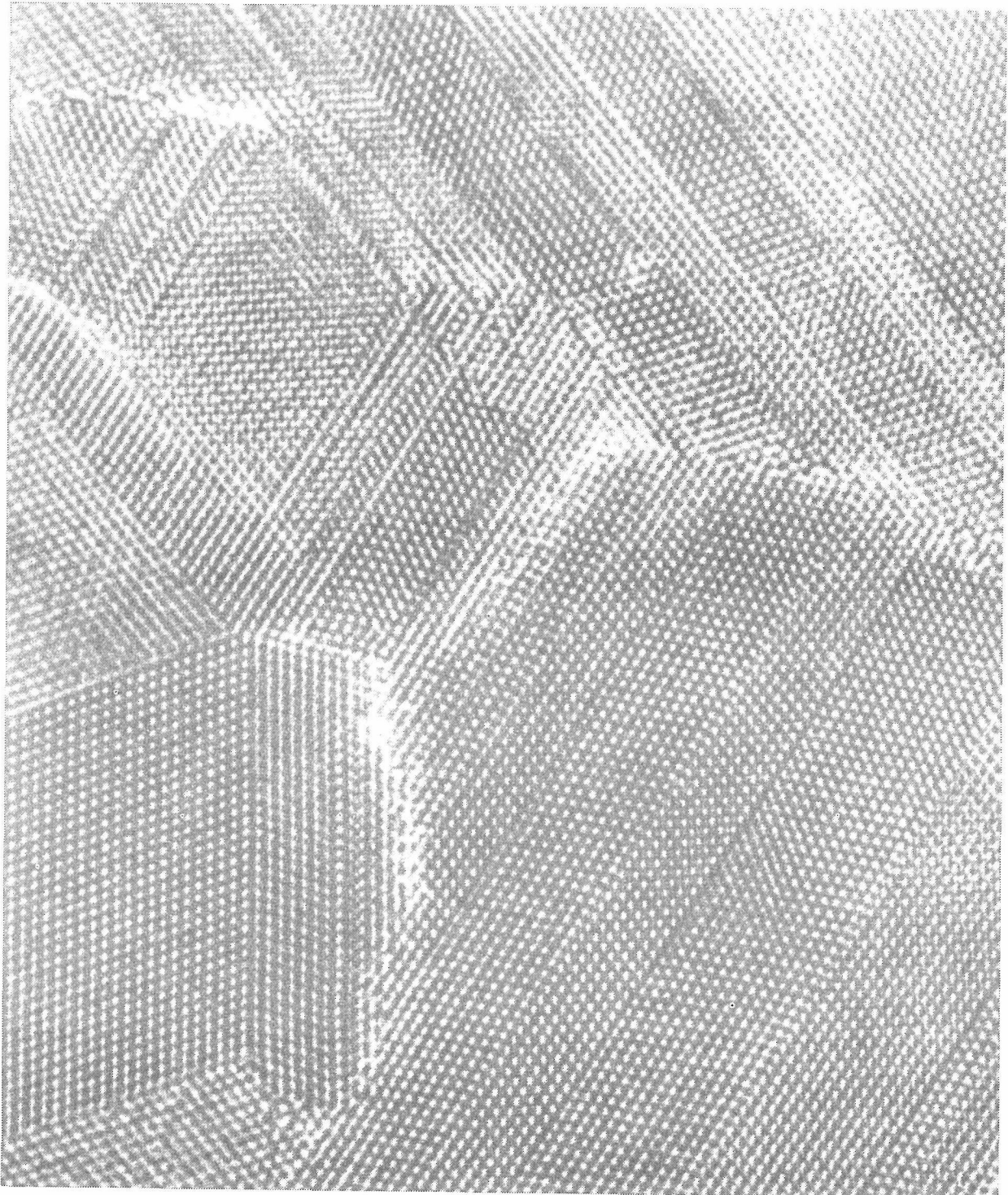
Fig. 3 Complex, high order boundary interactions in \langle 110 \rangle oriented grain of CVD diamond.
