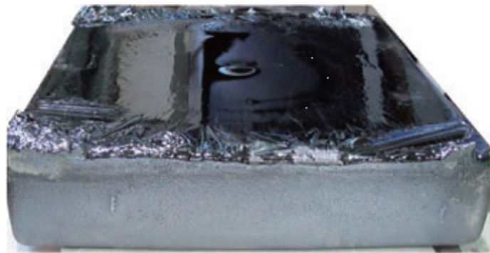
Figure: Photograph of the silicon ingot grown with the optimum conditions observed in the current study.
