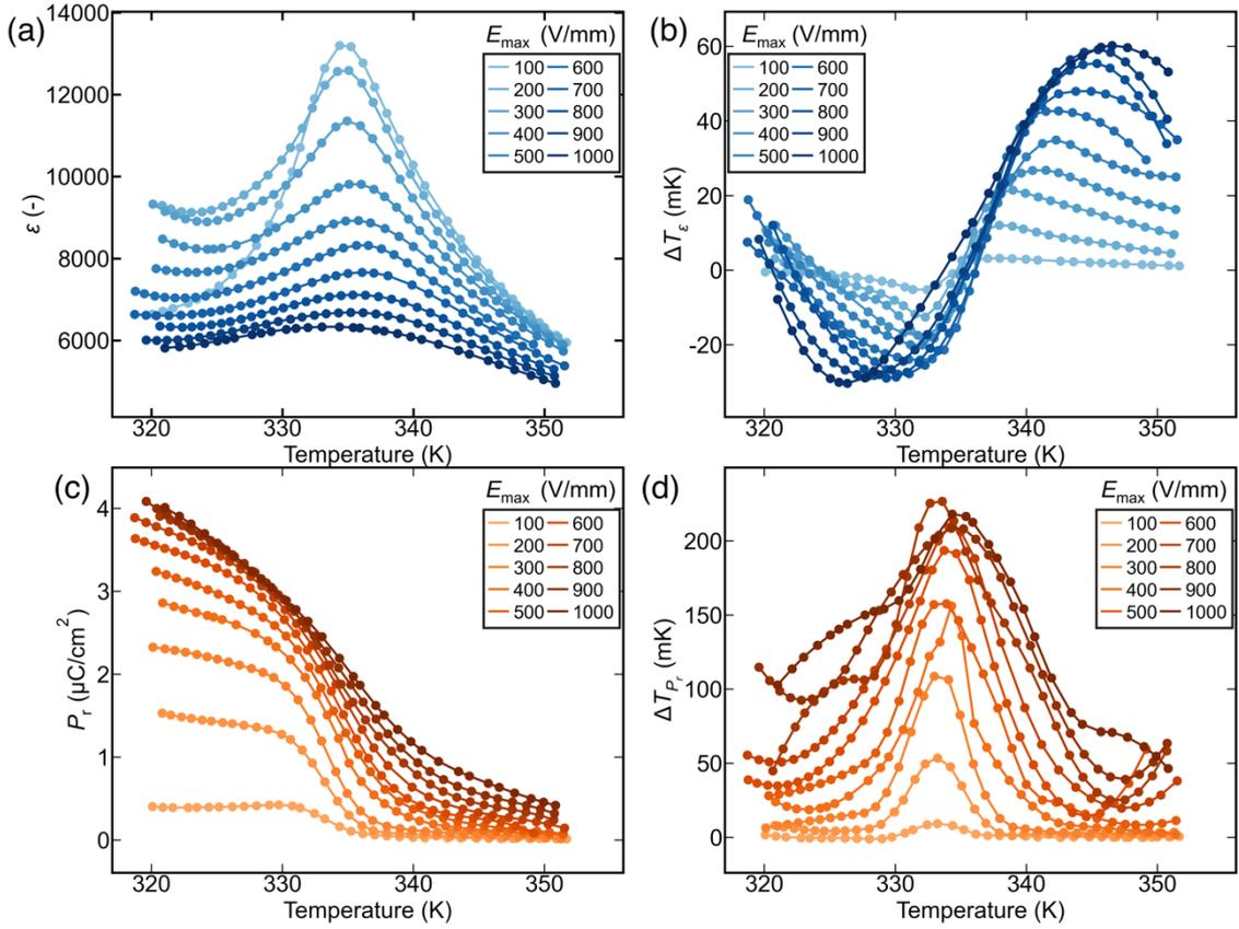
**Figure 3.**  $T$ -dependences of (a)  $\epsilon$ , (b)  $\Delta T_\epsilon$ , (c)  $P_r$  and (d)  $\Delta T_{P_r}$  at various  $E_{\max}$
