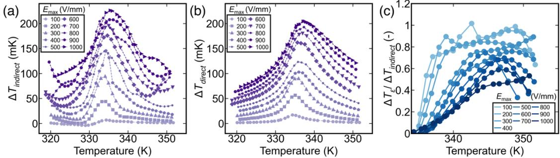
**Figure 4.**  $T$ -dependences of (a) the  $\Delta T_{\text{indirect}}$ , (b) the  $\Delta T_{\text{direct}}$  at various  $E_{\max}$  and (c) the  $\Delta T_\epsilon$  contribution ratio to the total  $\Delta T_{\text{indirect}}$  above the  $T_m$ .
