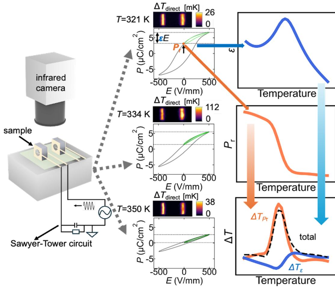
**Figure 1.** Experimental setup for LIT measurement and Sawyer Tower circuit. Thermal image,  $P$ - $E$  hysteresis and indirect  $\Delta T_{\text{Pr}}$ ,  $\Delta T_{\text{direct}}$  and overall  $\Delta T$  with temperature were incorporated into the figure.
