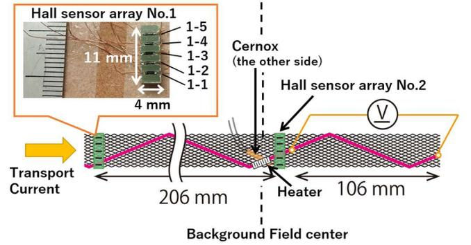
Fig. 3. Schematic of measurement setting. A heater for quench initiation is located at the background field center. One of two Hall-sensor arrays was equipped at 206 mm from a heater and close to a heater. The sensor HG-166A is 1.5 mm square, 0.6 mm in thickness.
