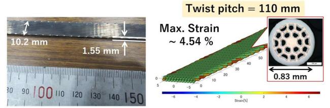
Fig. 1. Rutherford cable design result and the photo of the cable (after heat treatment). Maximum strain is around 4.5 % which is below the permissible one.
