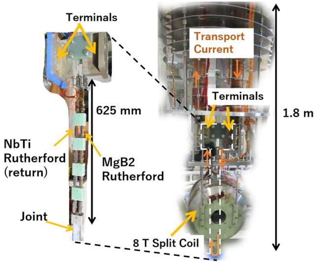
Fig. 2. The test device of Rutherford cable performance at NIFS.
