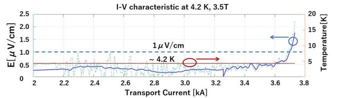
Fig. 4. Typical wave form of voltage runaway as a function of transport current. A solid horizontal line shown here is the temperature around the field center, which indicates the voltage occurrence was caused by over current under the field of 3.5 T.
