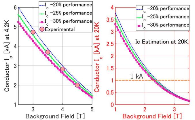
Fig. 5.  $I_c$  of the cable at various background fields. The curves at 20 K are the numerical estimations assuming the same deterioration observed at 4.2 K. Larger than 1 kA in 2 T field would be successfully expected.
