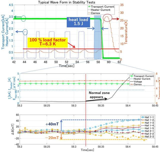
Fig. 6. Test result of quench initiation by heater current. The current re-distribution is observed by two hall-sensor arrays after normal zone appears.
