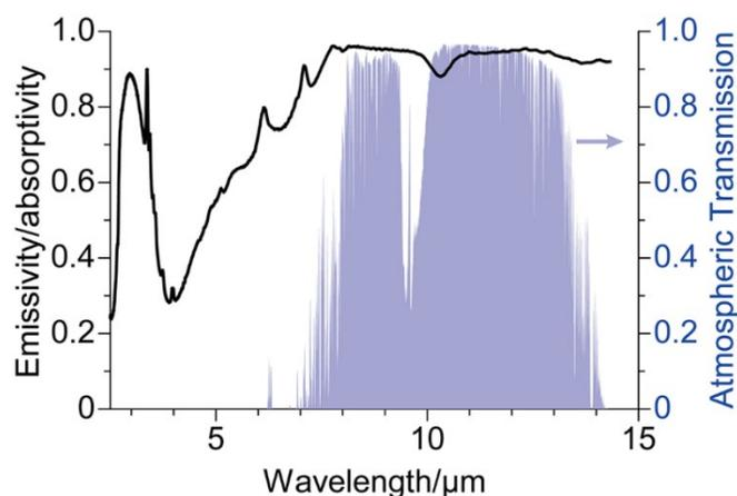
**Figure 6.** Emission/absorption spectrum of MG180 and the atmospheric window<sup>40</sup> in the mid-IR region.
