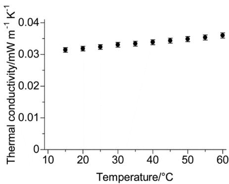
**Figure 5.** Thermal conductivity of MG180 measured by the HFM method.
