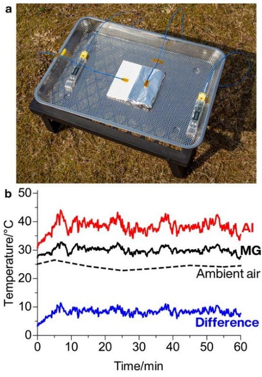
**Figure 4.** (a) Photograph of MG180/Al sample used for the solar radiation test. (b) Surface temperatures of MG180 and Al under sunlight and ambient air temperature. The blue line shows the temperature difference between Al and MG.
