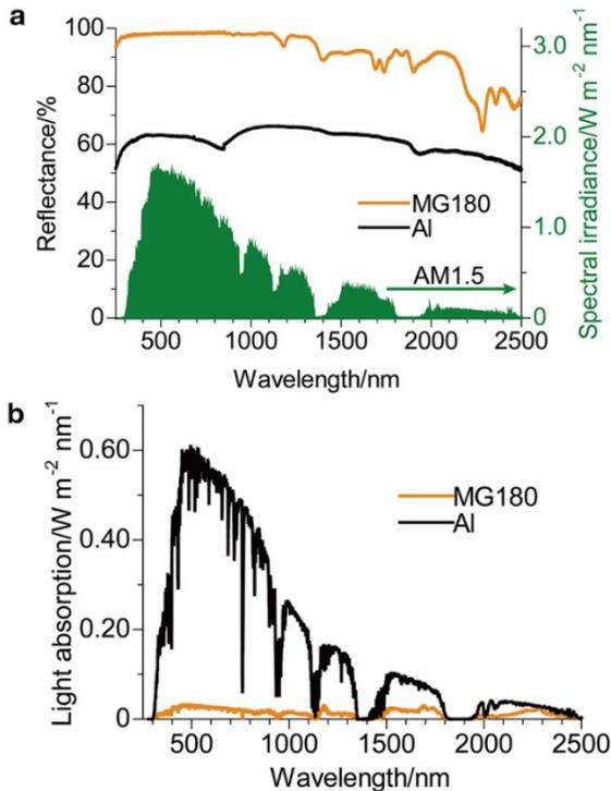
**Figure 3.** (a) Total light reflectance spectra of MG180 and Al, and AM1.5 (solar radiation).<sup>25,26</sup>
