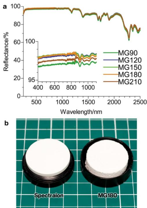
**Figure 2.** (a) Total light reflectance of MGs. (b) Photograph of Spectralon white reflectance standard and CNC-machined cylindrical MG180. Photograph during the machining is shown in FigureS6, Supporting information.
