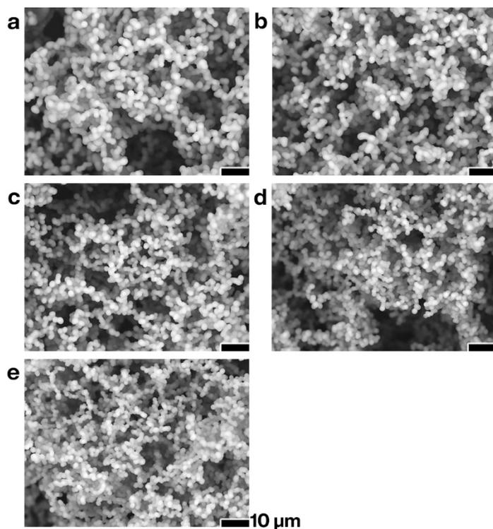
**Figure 1.** Scanning electron microscope (SEM) images of (a) MG90, (b) MG120, (c) MG150, (d) MG180, and (e) MG210.
