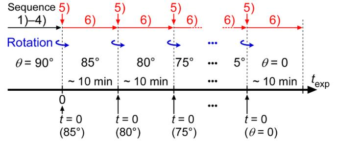
**Figure 2.** Schematic of the sequence for measuring the current decay by incrementally rotating the sample. In sequence (5), the sample is rotated by  $5^\circ$  within 1 s. At each angle,  $t$  is the elapsed time from when we started sample rotation. In sequences (6) and (7), we measured the current decay for approximately 10 min at each angle from 0 to  $85^\circ$ .
