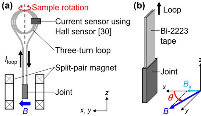
**Figure 1.** (a) Schematic of experimental setup. Horizontal magnetic field ( $B$ ) is applied to the joint using a split-pair superconducting magnet. The direction of magnetic field is controlled by rotating the sample. (b) Schematic showing the angle of magnetic field ( $\theta$ ). The perpendicular component of the magnetic field applied to the tape surface is  $B_x (=B \cos\theta)$ .
