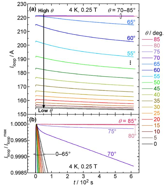
**Figure 4.** Time dependence of (a)  $I_{\text{loop}}$  and (b) normalized  $I_{\text{loop}}$  at 4 K, 0.25 T, and  $0-85^\circ$ .  $I_{\text{loop}}$  values are calculated using  $V_{\text{Hall}}$  values shown in figure 3. At angles less than  $70^\circ$ ,  $I_{\text{loop}}$  at 600 s decreases as the angle decreases owing to a decrease in  $I_{\text{cj}}$ . A persistent current continues to flow in the sample at high angles of  $75-90^\circ$ .
