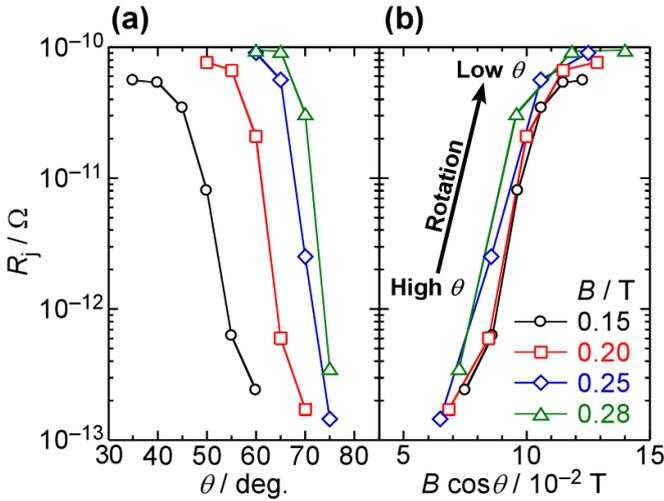
**Figure 7.** (a) Sections of  $R_j$  in region (ii) of figures 5(a)–(d). Region (ii) shifts toward higher angles as the magnetic field increases. (b) Relationship between  $B \cos \theta$  and  $R_j$  in region (ii). The significant changes in  $R_j$  at each magnetic field are nearly identical at  $B \cos \theta$  of  $6\text{--}11 \times 10^{-2}$  T, which are independent of the magnitude of the magnetic field.
