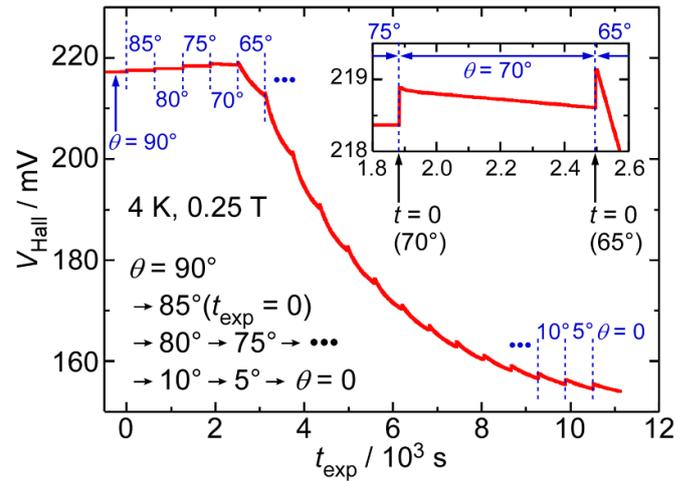
**Figure 3.** Voltage of Hall sensor ( $V_{\text{Hall}}$ ) in the current sensor as a function of experimental time ( $t_{\text{exp}}$ ) at 4 K and 0.25 T. We started to rotate the sample from  $90^\circ$  at  $t_{\text{exp}} = 0$  by  $5^\circ$  within 1 s. Inset shows a magnified view at approximately  $70^\circ$ .
