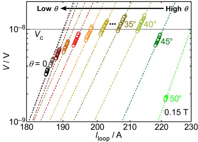
**Figure 6.** Smoothed  $V-I_{\text{loop}}$  curve at 0.15 T and 0–50°.  $V-I_{\text{loop}}$  at 0–50° is fitted to the power law model, as shown by dashed lines.
