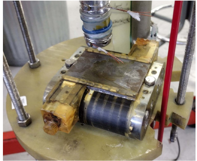
Figure 6. Picture of the first TELENE impregnated Nb 3 Sn small undulator attached to its test insert.
