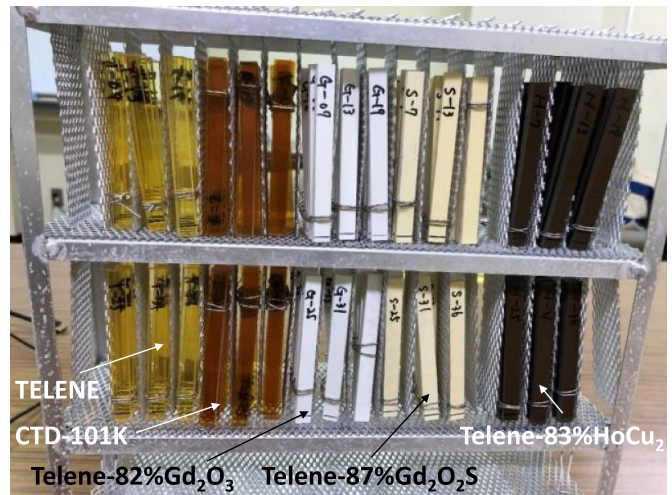
Figure 7. Picture of aluminum crate containing the resins to be gamma ray irradiated in air atmosphere.
