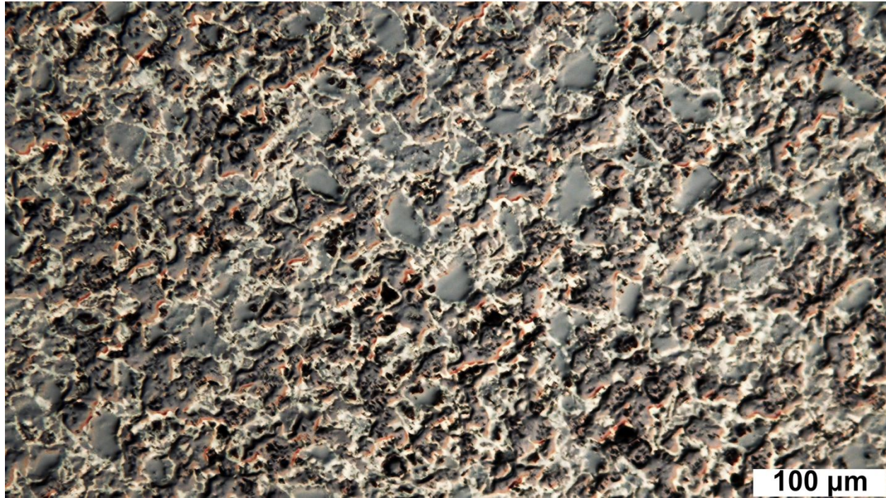
26 27 28 29 30 31 Figure F5. Structure of the multiboride ceramic composite after spark plasma sintering at 1900 °C by an optical microscope. Chain-cell structure can be observed.
