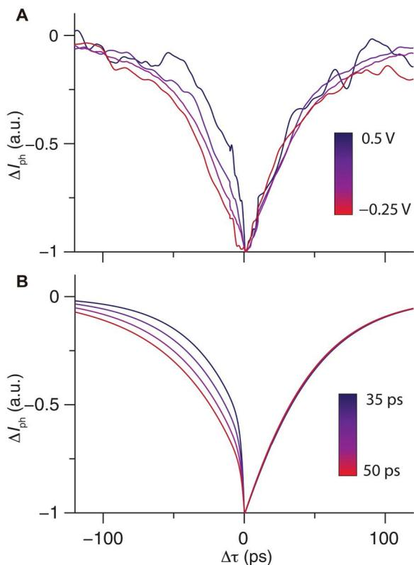
**Fig. 4. Pump-probe photocurrent measurement in the 4L region.** (A) Bias-dependent pump-probe photocurrent measurement in the 4L region with bias voltages ranging from  $-0.25$  to  $0.5$  V. The measurements are carried out with an IR-pulse (VIS-pulse) fluence of approximately  $350(2)$   $\mu\text{J cm}^{-2}$ . (B) Numerical modeling results with the response time of the slow component varying from 35 to 50 ps.
