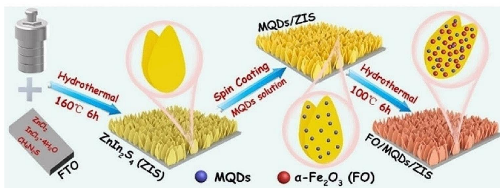
Fig. 6 Process for photoelectric conversion devices; monodisperse MXene quantum dots were obtained by HF etching, exfoliation, and hydrothermal treatment; next, ZnIn 2 S 4 nanosheet arrays were synthesized on FTO by hydrothermal method; then, MXene quantum dots
