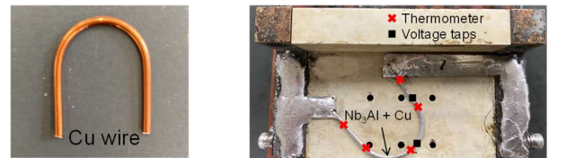
Fig. 11. Photographs of the pre-bended copper wire and sample stage to measure the bending strain characteristics of Type D wire.
