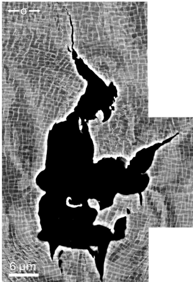
Fig. 16—Stitched SEM-ECCI of \langle 001 \rangle oriented CMSX-4 tested at 800\text{ }^{\circ}\text{C}/10^{-4}\text{ s}^{-1} showing cracks growing from pores perpendicular to the loading direction.
