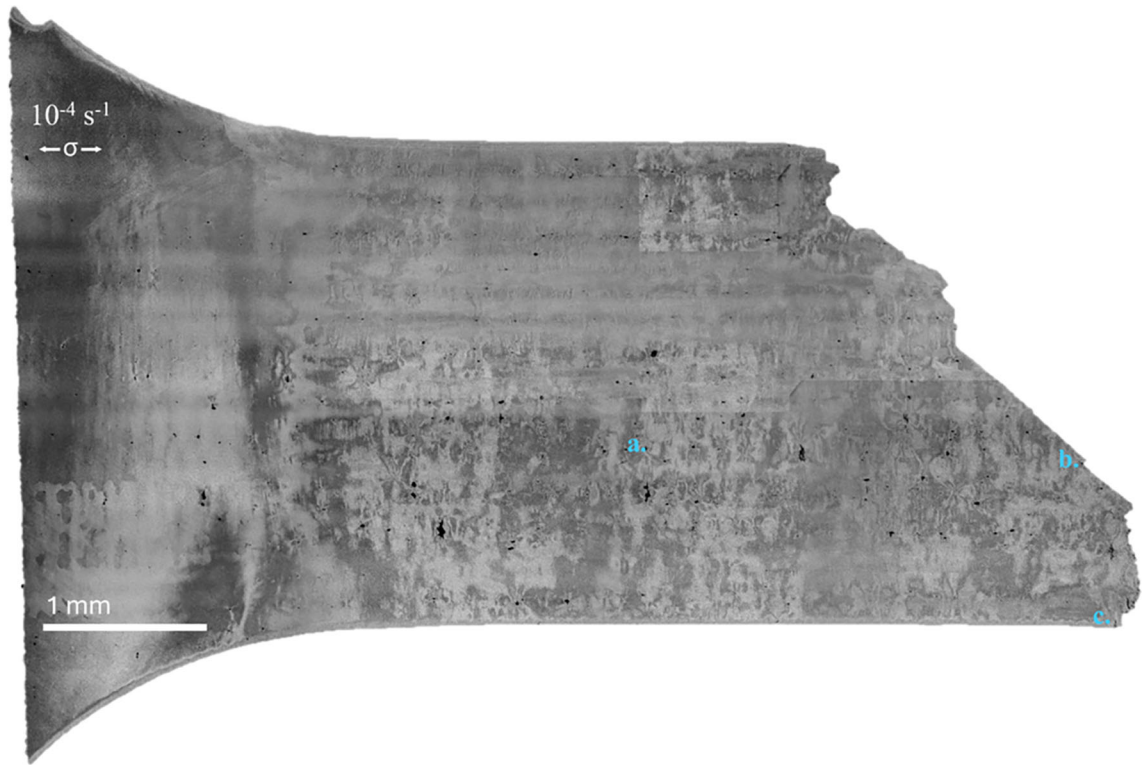
Fig. 12—Stitched SEM-ECCI image of the gauge section, observed near the (110) plane, after failure for the 800 °C/ 10^{-4} \text{ s}^{-1} condition.
