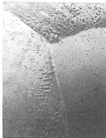
Fig. 27 A micro-slope on the ( \bar{1}\bar{1}\bar{1} ) nitrogen surface of cBN and its etching pattern by the LiCaBN 2 flux.
