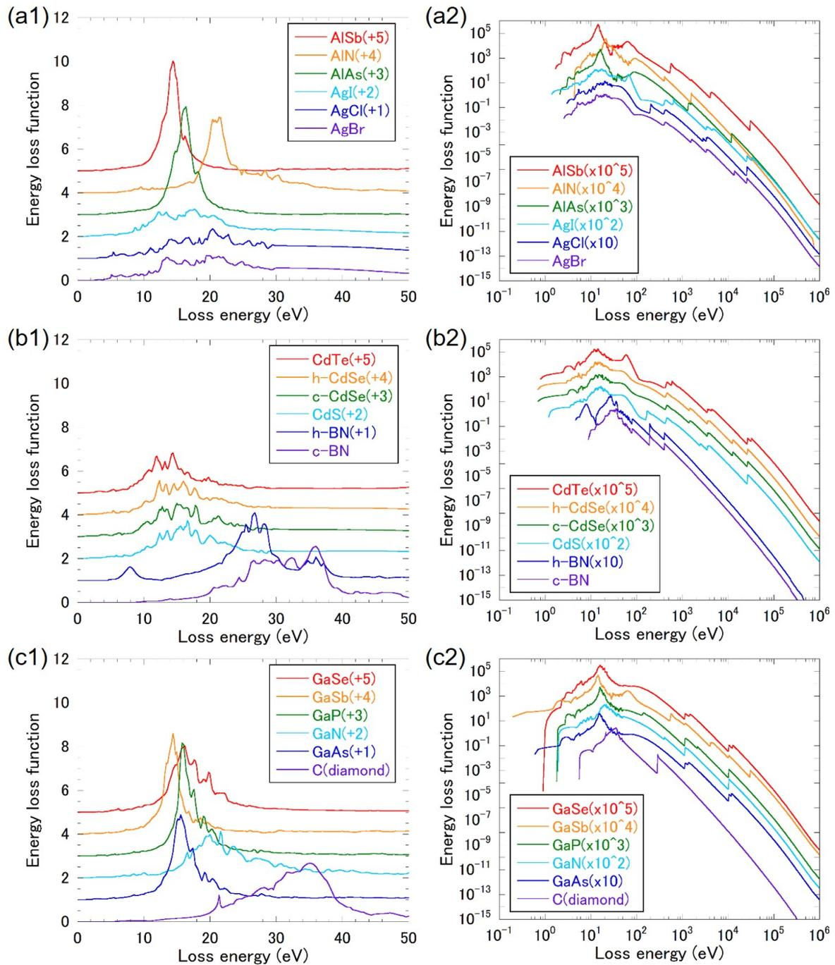
Figure 2: Energy loss functions for the 35 materials in this study. Lefthand figures are bilinear plots, and righthand figures are log-log plots. The vertical axis is shifted for each material to avoid overlapping of each graph.
