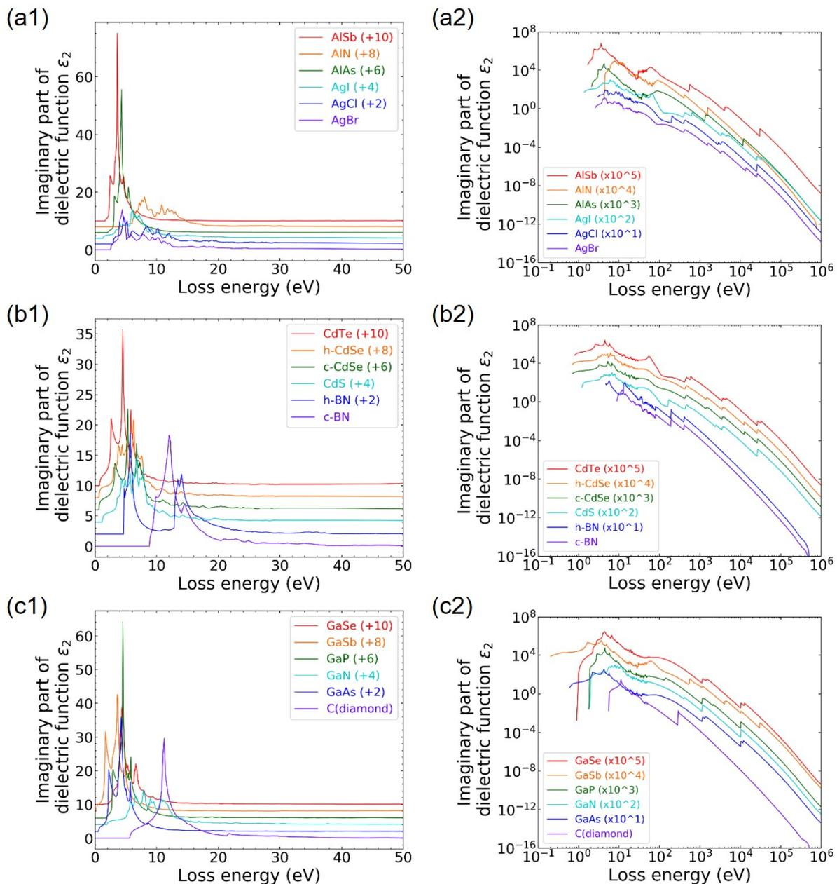
Figure 6: Energy loss functions for the 35 materials in this study. Lefthand figures are bilinear plots, and righthand figures are log-log plots. The vertical axis is shifted for each material to avoid overlapping of each graph.
