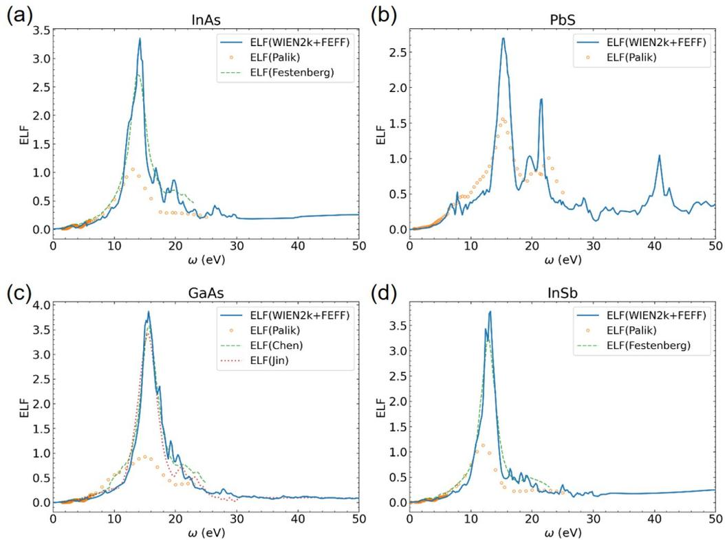
**Figure 7:** Plots of energy loss functions (ELFs) for (a) InAs, (b) PbS, (c) GaAs, and (d) InSb. Blue solid lines represent ELFs calculated by WIEN2k and FEFF. Orange open circles represent ELFs from the optical data tabulated by Palik [12–14]. Green dashed line represents the ELF measured by Festenberg *et al.* [31] or the ELF as analyzed by Chen *et al.* [32].
