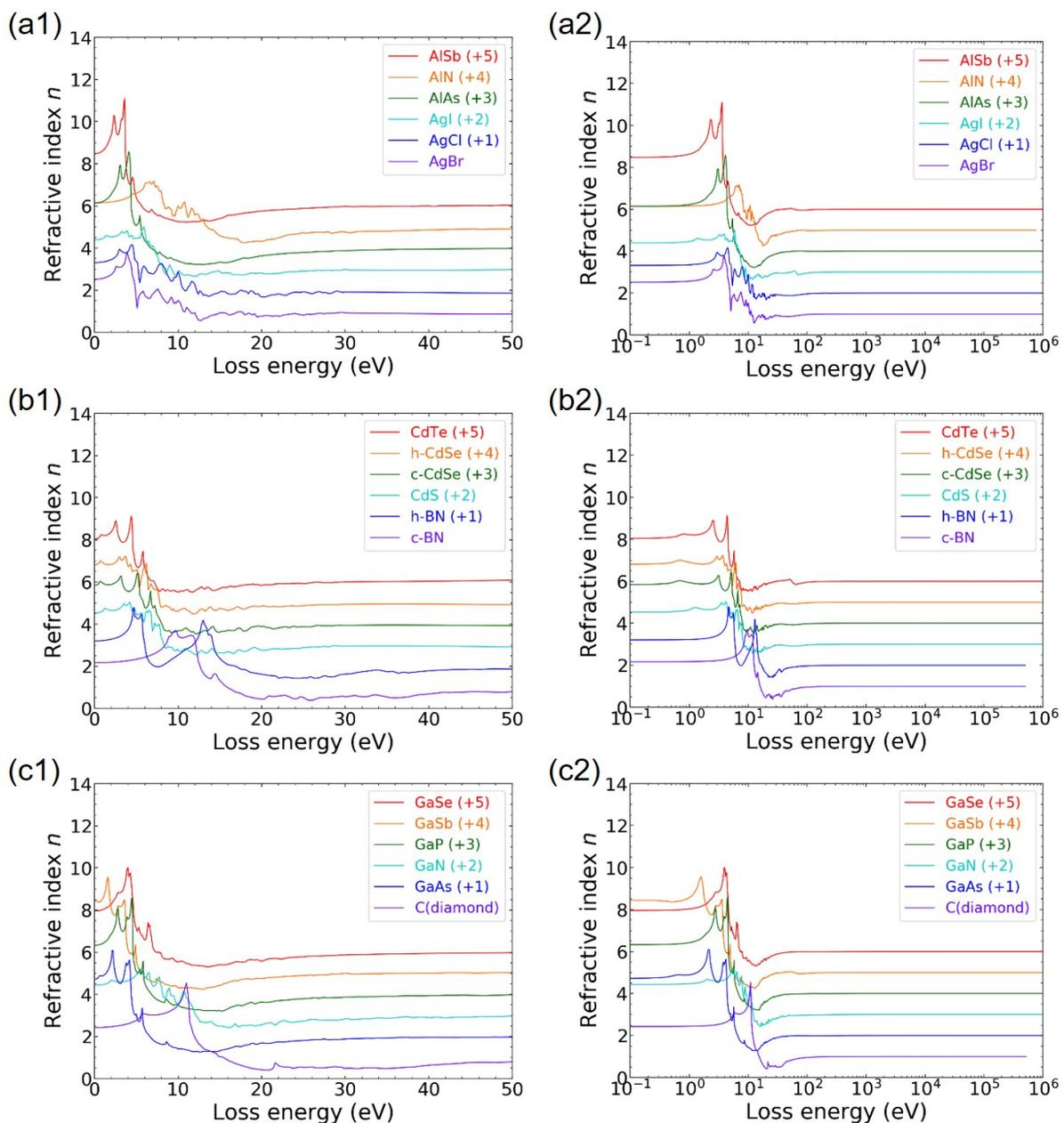
**Figure 3:** Refractive indexes for the 35 materials in this study. Lefthand figures are bilinear plots, and righthand figures are log-linear plots. The vertical axis is shifted for each material to avoid overlapping of each graph.
