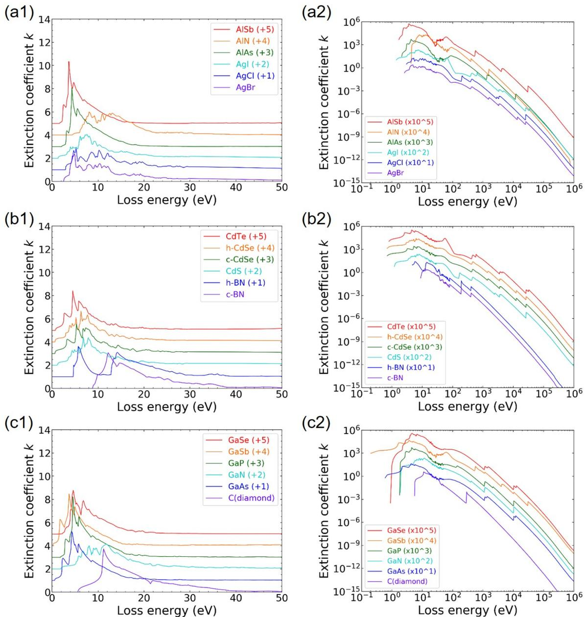
Figure 4: Extinction coefficients for the 35 materials in this study. Left-hand figures are bilinear plots, and right-hand figures are log-log plots. The vertical axis was shifted for each material to avoid overlapping of each graph.
