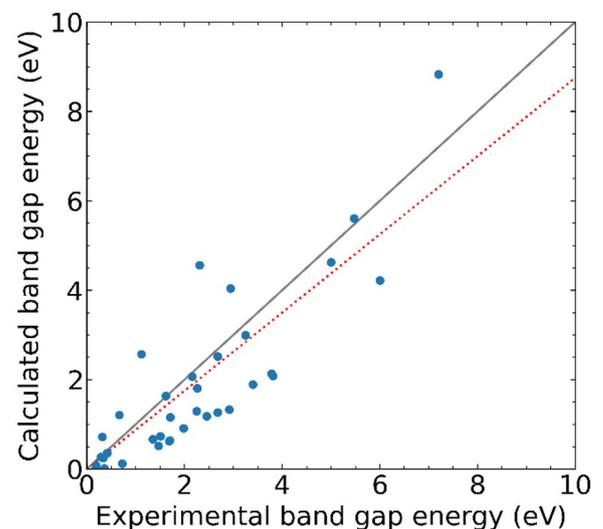
**Figure 8:** Comparison of calculated band gap energies with experimental values. Solid line represents the case where the measured and calculated band gap values are equal. Dotted line indicates the curve fit result.
