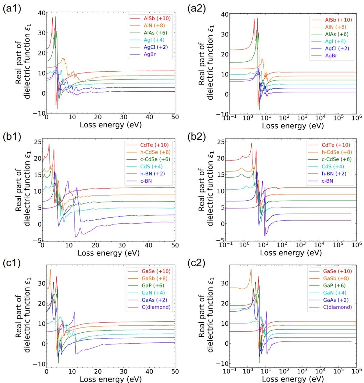
**Figure 5:** Real part of the dielectric functions for the 35 materials in this study. Left-hand figures are bilinear plots, and right-hand figures are log-linear plots. The vertical axis is shifted for each material to avoid overlapping of each graph.
