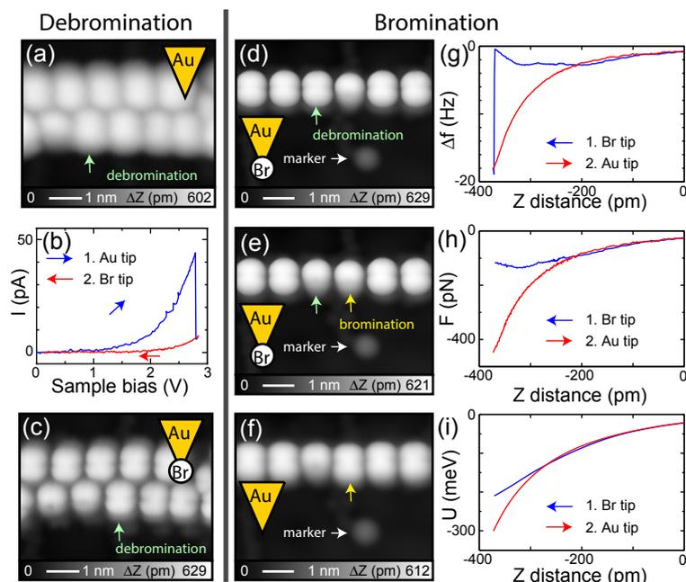
**Fig. 5.** (a) STM topography taken before the debromination. (b)  $I$ - $V$  curve taken during the debromination. (c) STM topography after the debromination. (d-f) Bromination reaction by the local probe. (g) Frequency shift curve measured during the addition reaction, (h) the extracted force and (j) potential curves.
