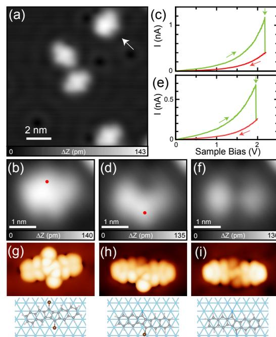
**Fig. 2.** (a) STM topography of the precursor molecules adsorbed on Cu(111) and (b) the close-up view. (c)  $I$ - $V$  curve measured during the debromination reaction. (d) STM topography after the debromination. (e)  $I$ - $V$  curves measured during the second debromination reaction. (f) STM topography after the second debromination. (g–i) Simulated STM topographies and their adsorption geometries.
