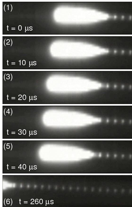
Fig. 4. Ultrahigh-speed photographs of fiber-fuse propagation for the 9 W condition. The view is the same height as that of Fig. 3(2-a).
