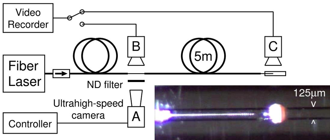
Fig. 1. Experimental setup and a captured video image of fiber-fuse ignition taken from camera C.
