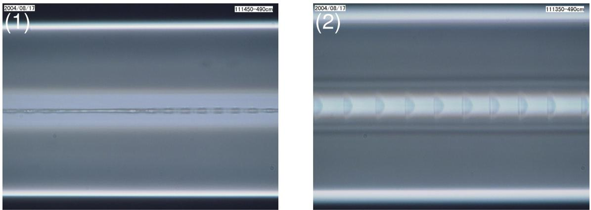
Fig. 5. Optical microscope images of the fiber-fuse damage. The voids on the right appear at intervals of about  $23 \mu\text{m}$ , which is in good agreement with that for the scattering points shown in Fig. 4.
