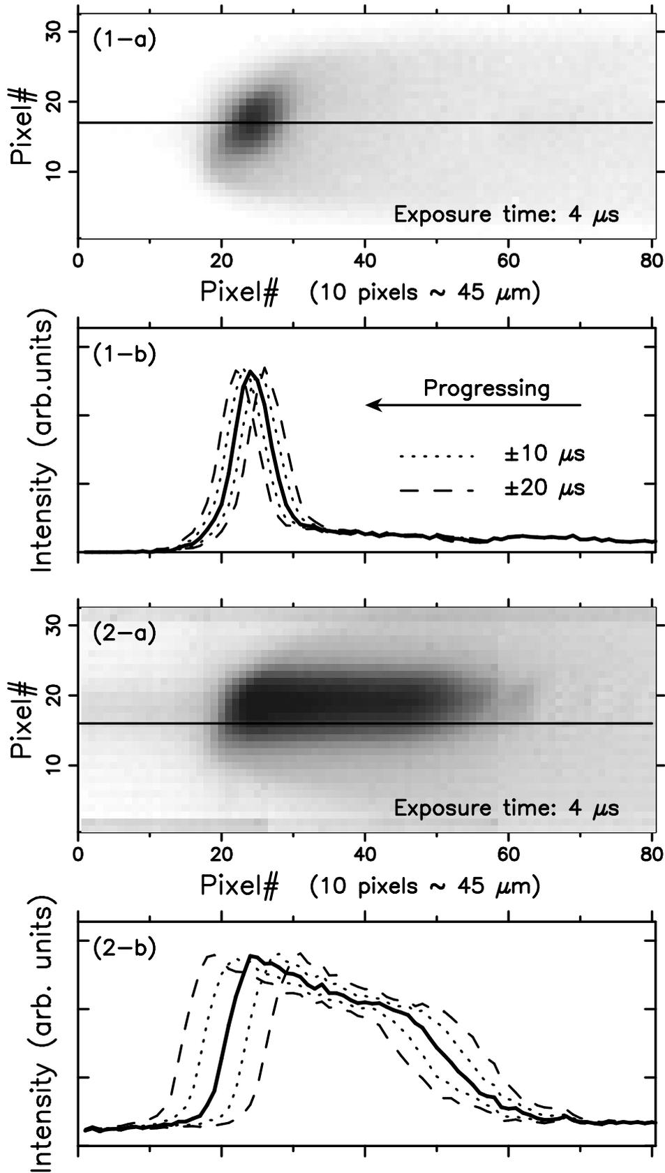
Fig. 3. Photographs of fiber-fuse propagation from the camera A (1-a & 2-a) and intensity profiles along the black lines on the photos for 5 successive frames (1-b & 2-b). The intensities of the laser ( $\lambda=1480$  nm) coming from the left were about 2 W (1) and 9 W (2).
