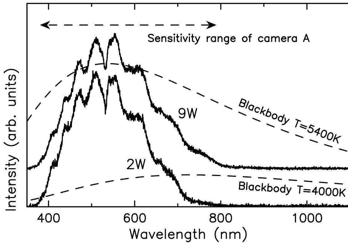
Fig. 2. Emission spectra of the optical discharge measured near camera B. Their intensities are normalized so as to be equal in height. The horizontal arrow indicates the sensitivity range of ultrahigh-speed camera A. The dashed lines are theoretical spectra of blackbody radiation at 5400K and 4000K.
