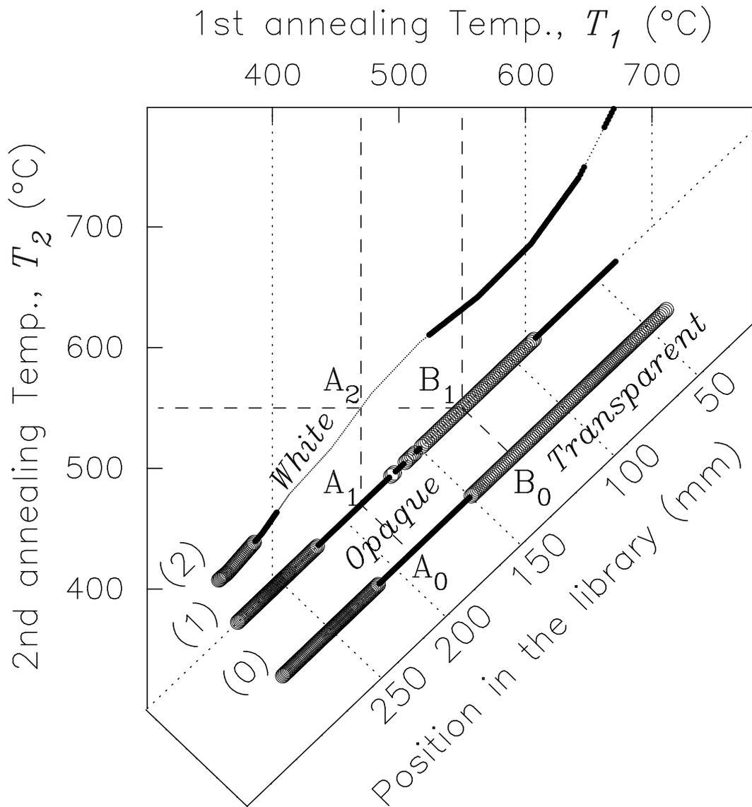
Fig. 3. Annealing condition of the sample libraries and appearance of the annealed glass segments inside. (0) with no annealing treatment for reference. (1) with 1st annealing for 5min only. (2) with two successive heat treatments, each for 5min. Thick line plotted by  $\circ$ : completely transparent segment, thin line by  $\cdot$ : white, and medium line by  $\bullet$ : opaque(see text).  $A_n$  and  $B_n$  indicate specific glass segments. These notations are also used in Fig. 4 and Fig. 5.
