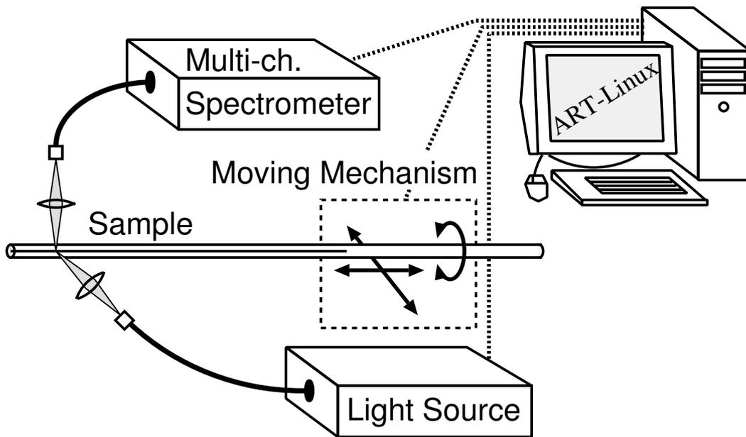
Fig. 2. The fluorescence lifetime measuring equipment used in this study(see text).
