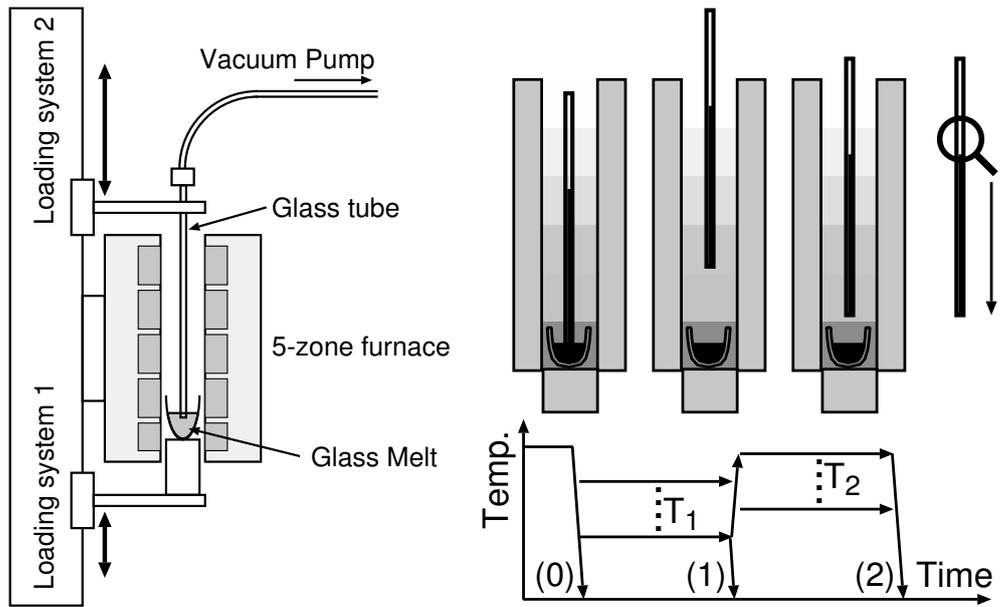
Fig. 1. (a: left) The structure of vertical temperature gradient furnace used in this study and (b: right) an illustration showing 2-step annealing procedure(see text).
