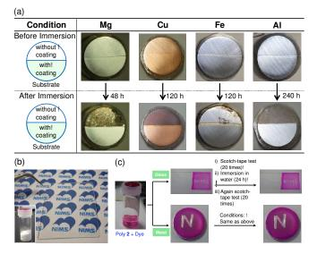
Fig. 6 (a) Visual appearance of half-circle coated various substrates before and after immersion in salt water for specified time in hours. Plates were 15 mm in
