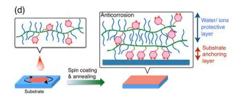
**Fig. 1** (a) Photograph of a blue mussel and its adhesive byssus, which contains mainly catechol and amine (dopamine) units. (b) Chemical structure of poly(dopamine methacrylamide-*co*-alkyl methacrylate), poly(DOMA-*co*-AMA). (c) Various combinations, compositions, and gel permeation chromatography (GPC) data of poly **1-3**. (d) Schematic illustration of preparing ultrathin polymer coating and possible pathway of forming stable protecting layer on metal/alloy substrates.
