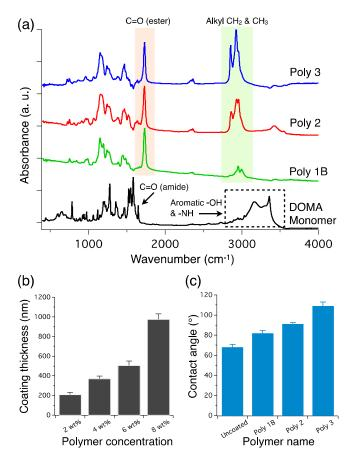
Fig. 3 (a) FT-IR spectra comparison of dopamine methacrylamide (DOMA) monomer and different polymers in KBr pellet. (b) Relation between polymer concentration and thin-film thickness measured by surface profiler. (c) Static water contact angle comparison of different polymer coated metal substrates at 298 K.
