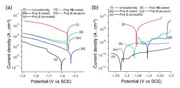
Fig. 5 (a) Cathodic, and (b) anodic polarization curves of uncoated/polymer coated Mg alloy (AZ31) substrate after 1 h immersion in 3.5 wt.% aqueous NaCl solution at 298 K (scan rate 1 mV/s).
