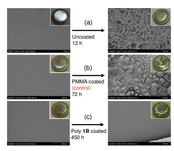
Fig. 7 SEM images of (a) uncoated, (b) PMMA coated, and (c) poly 1B coated Mg substrates before and after hydrogen evolution test at 298 K. Inset images are respective resin embedded samples.
