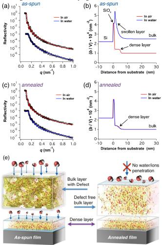
**Fig. 8** Neutron reflectivity for (a) as-spun and (c) annealed films in air and water. Open symbols depict experimental data, and solid lines represent the reflectivity calculated on the basis of the scattering length density (b/V) profiles shown in (b, d). For clarity, the values in panel (a, c) are offset from one another. (e) Schematic illustration of difference between as-spun and annealed film determined by neutron reflectivity measurement.
