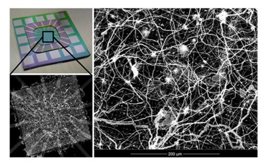
Figure: A look inside the ASN device reveals its highly interconnected architecture which comprises synaptic circuit elements at each point of contact between nanowires. The collective interactions between these atomic switches result in unique, emergent properties which have shown significant potential for neuromorphic computing.
