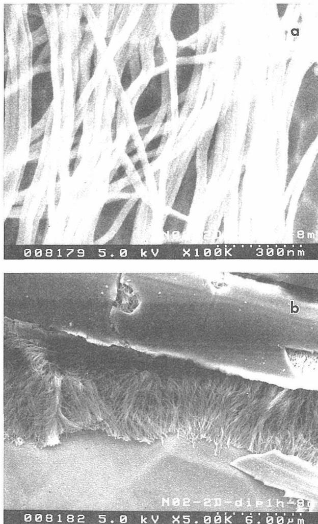
図3.1 High magnification SEM (a) and low magnification SEM (b) images of Silicon oxide nanofibers obtained by immersing the ordered anodic alumina for 1min in the sol which is aged at room temperature for 2days.
