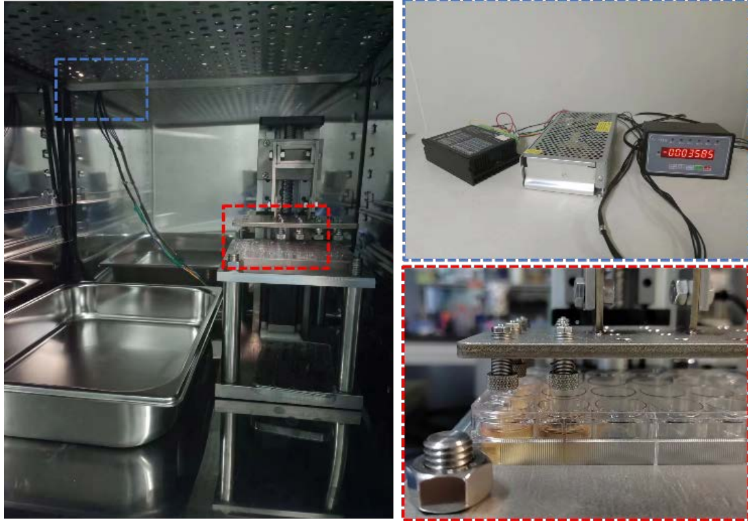
Figure S10. The bioreactor with cyclic compression function. In the blue frame is the external drive motor of the compression unit. In the red box is compression device applying pressure to the scaffold in the cell culture plate.
