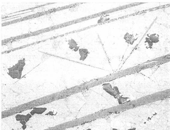
Fig. 1 Scanning electron micrograph for the arc melted YPd_5B_3C_{0.5} ingot. The 23 K superconducting phase is embedded as plate like crystals in the matrix of other phases.
