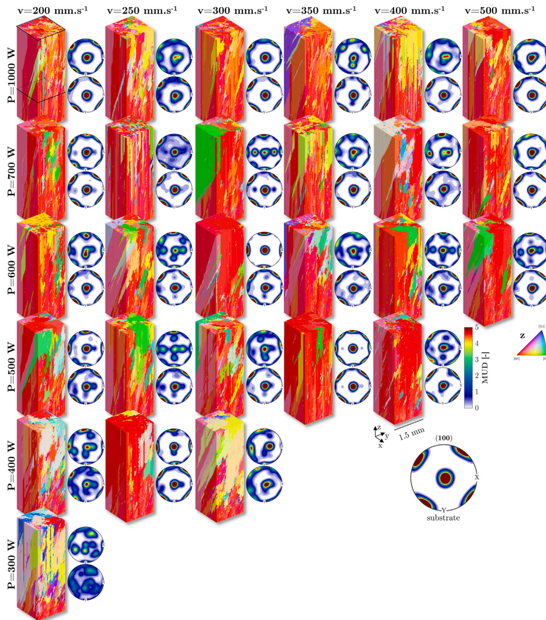
Fig. 10. Numerical microstructures predicted by CA with a nucleation density N_0 = 10 \times 10^{12} \text{ m}^{-3} and corresponding (100) pole figures in the XY plane at two different build height for the different build conditions. The IPF color coding is along the z-direction.
