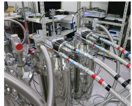
Figure 2. Photo of two G-M cold heads and vacuum chambers.
